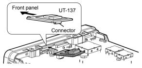
Carefully, push the connector into the socket.
