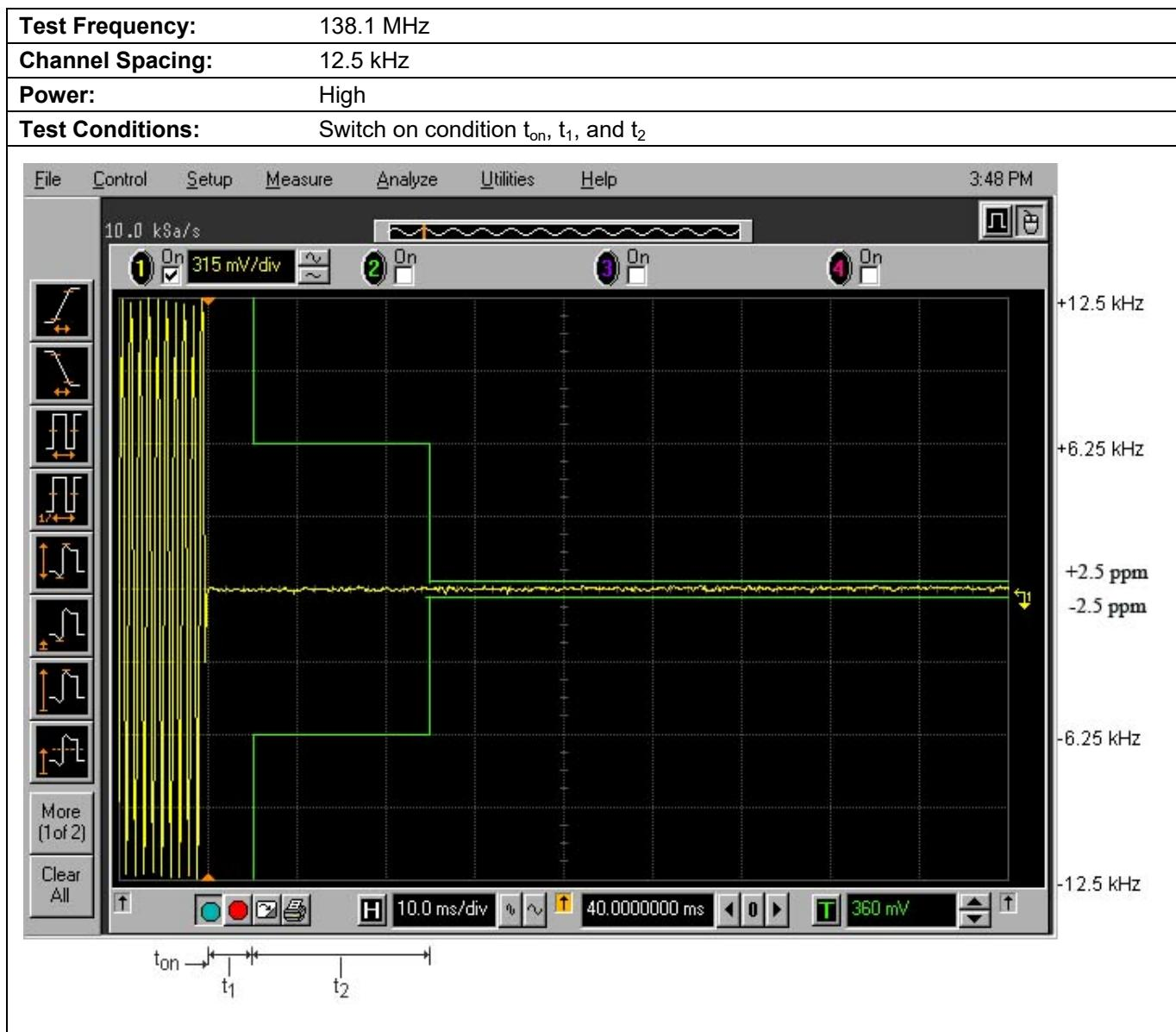
**Plot 4.12.3.2. Transient Frequency Behavior for 12.5 kHz Channel Spacing**
