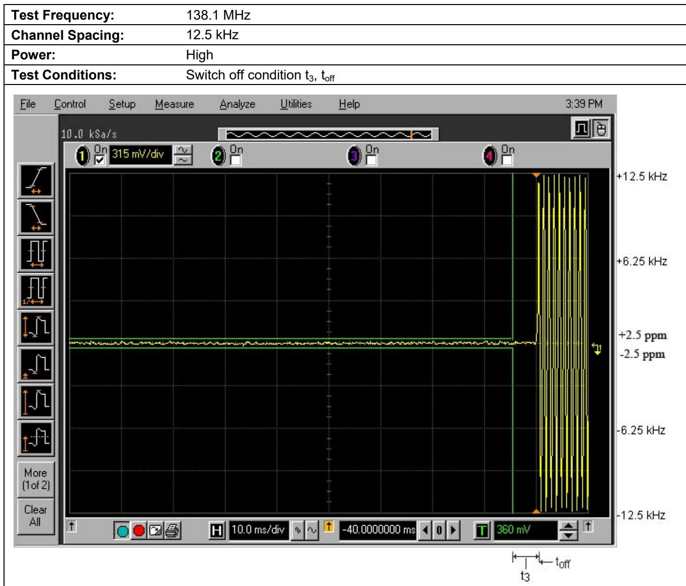
**Plot 4.12.3.3. Transient Frequency Behavior for 25 kHz Channel Spacing**
