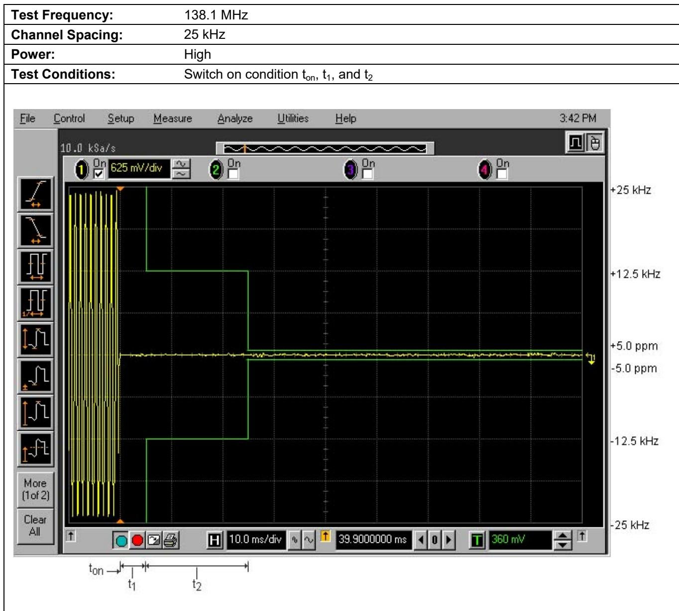
**Plot 4.12.3.4. Transient Frequency Behavior for 25 kHz Channel Spacing**
