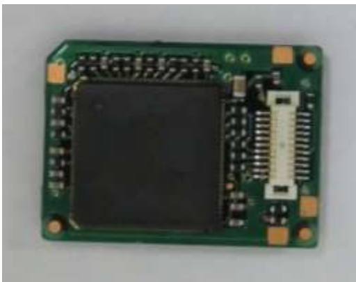
IC-F7510 AES/DES UNIT (UT-125 FIPS) SIDE B
