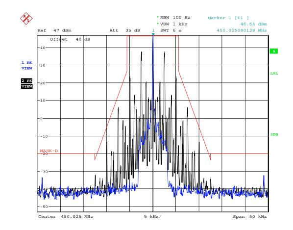
5.8.3.1.19. Configuration: Mask D, 450.025MHz, 12.5 KHz, Analog, High power
