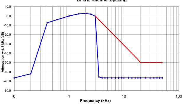
Audio Frequency Response 25 kHz Channel Spacing
