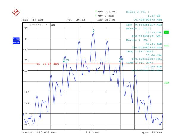
*5.8.3.1.1. Configuration: 99% OBW, 450.025MHz, 12.5 KHz, Analog, High power* OBW: 10.497 KHz
