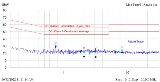
Peak QP Qp-Qp Limit Avg Avg-Avg Limit **Trace Name** Frequency dBuV dB MHz dBuV dBuV dB 0.749 33.7 30.8 -25.2 28.9 -17.1 Return Trace
