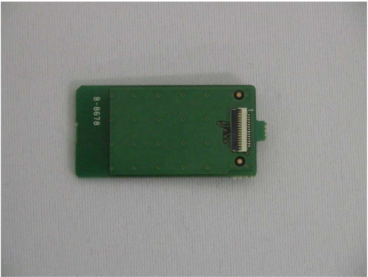
IC-F7520 RELAY-A UNIT A SIDE
