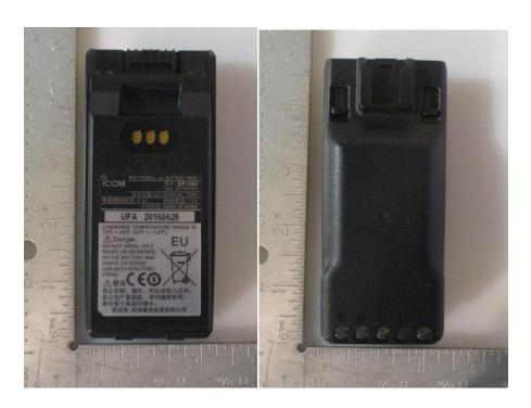
Li-ion Chargeable Battery (M/N: BP-284 Li-ion, 7.2V, 3210mAh)
