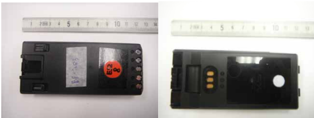
Li-ion Chargeable Battery (M/N: BP-283 Li-ion, 7.2V, 2010mAh)
