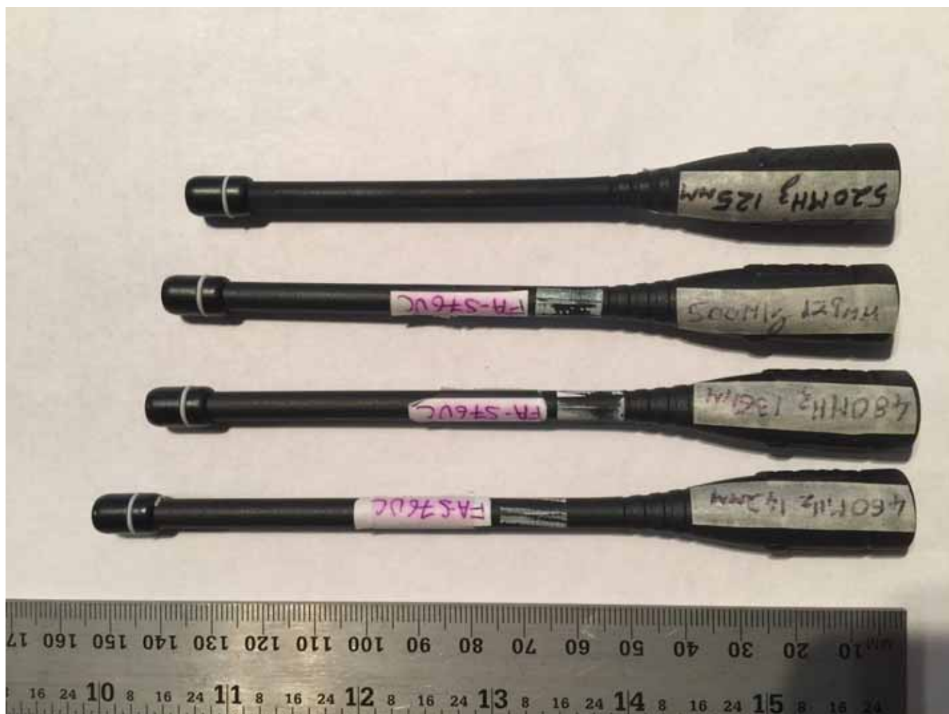
< FA-S76UC Cut Antenna >
