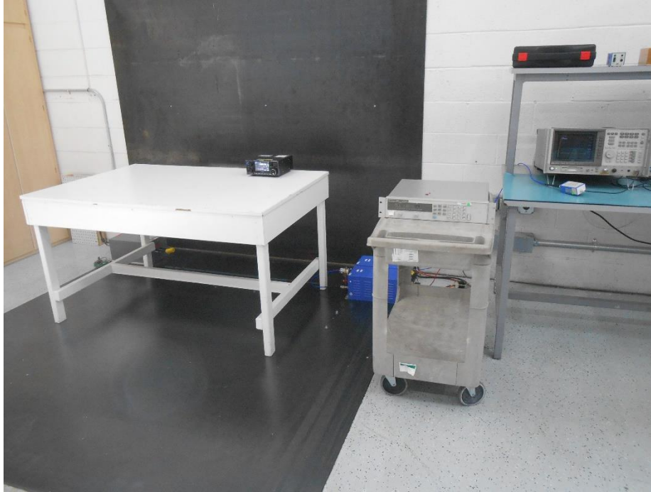
DC Conducted Emissions Test Setup Photo
