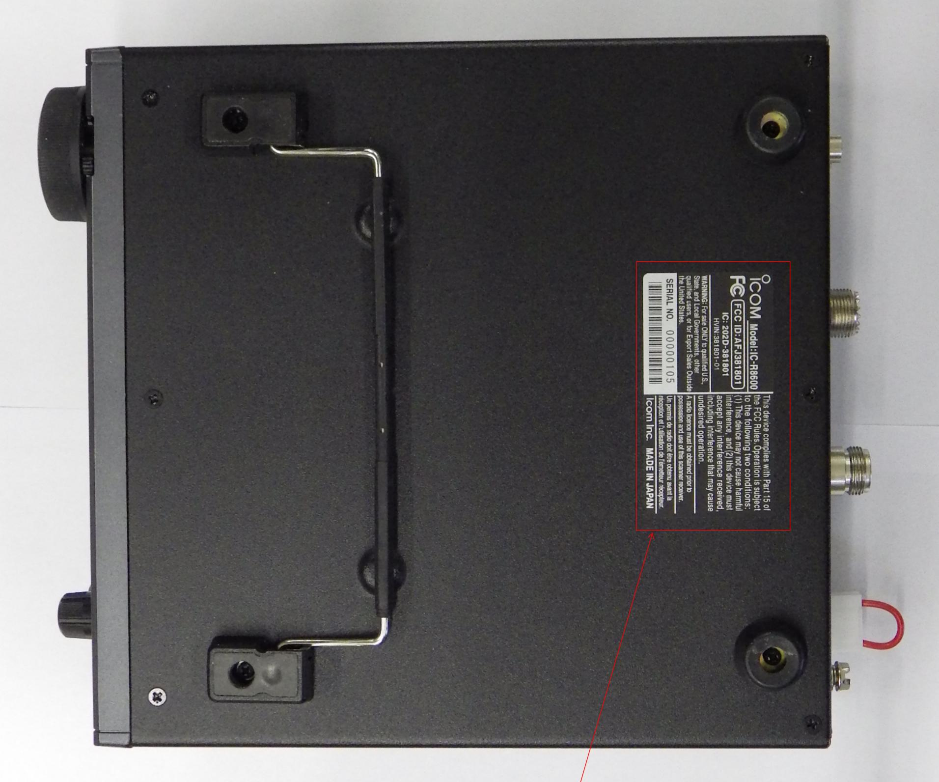
Serial seal is attached here.
