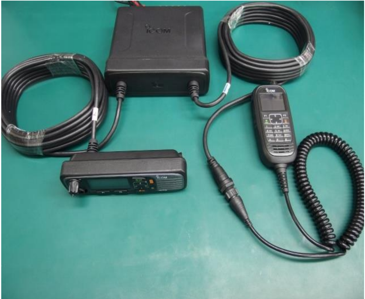
Radio body + separation kit (RMK5) + remote head (RMK5) + remote microphone (HM-218)
