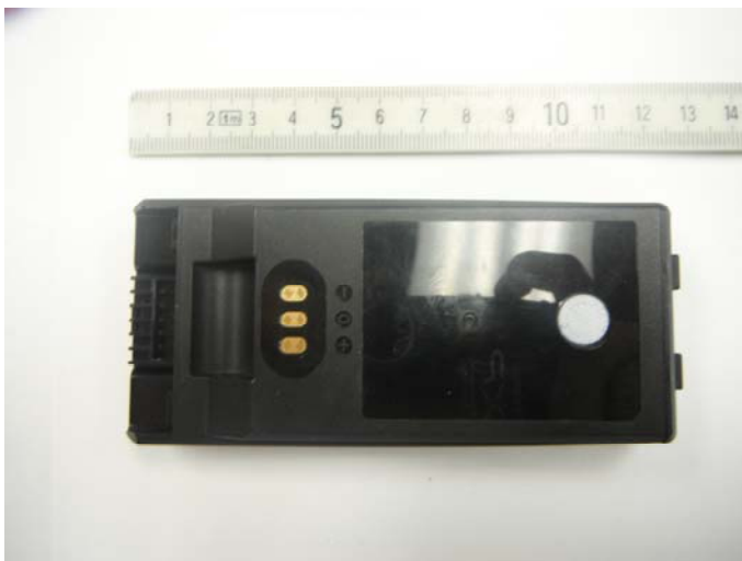
Li-ion Chargeable Battery (M/N: BP-285 Li-ion, 7.2V, 3210mAh)
