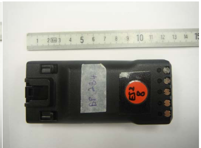
Li-ion Chargeable Battery (M/N: BP-285 Li-ion, 7.2V, 3210mAh)
