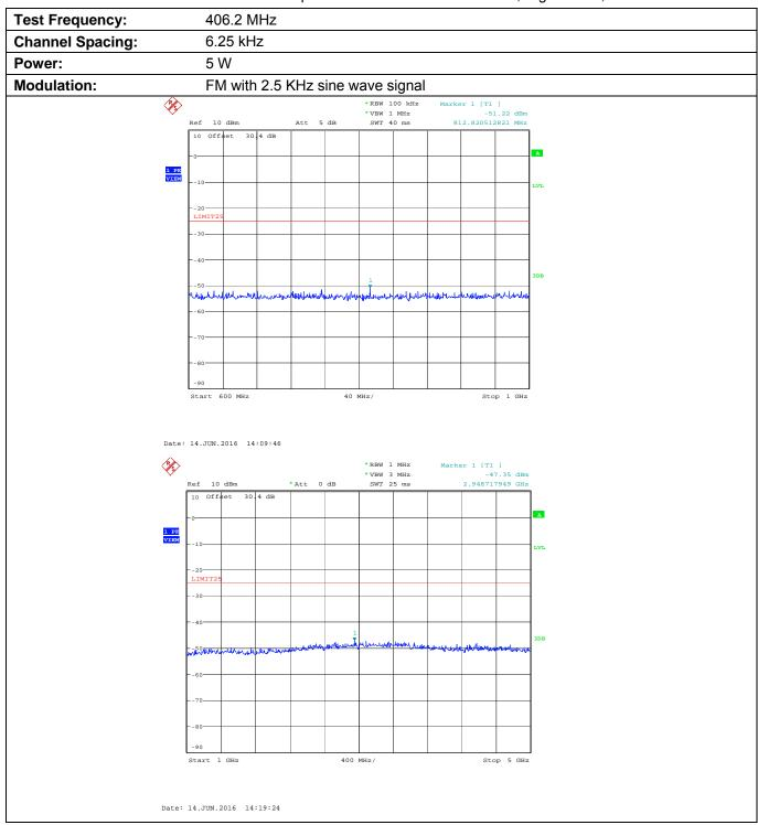
Plot 5.9.4.1.3. Conducted Transmitter Spurious Emissions for 406.2 MHz, Low Power, 30 MHz - 600 MHz
