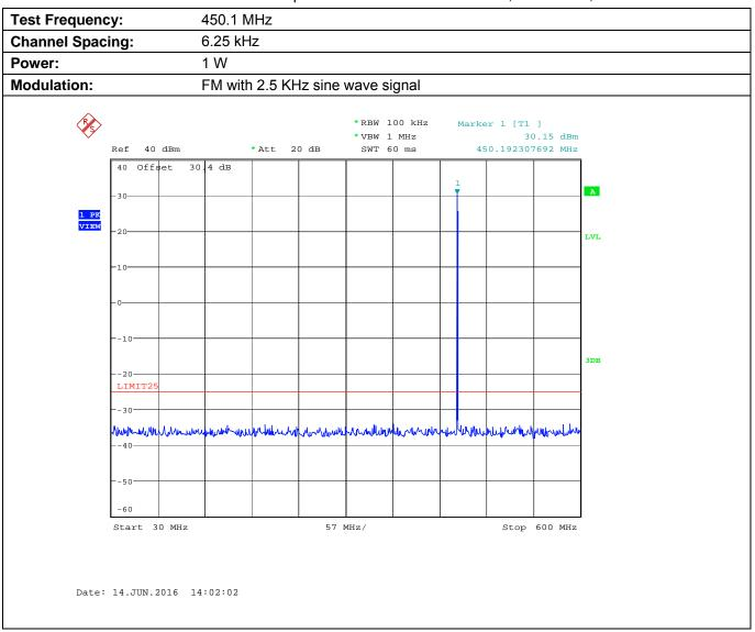
Plot 5.9.4.2.4. Conducted Transmitter Spurious Emissions for 450.1 MHz, Low Power, 600 MHz – 5 GHz
