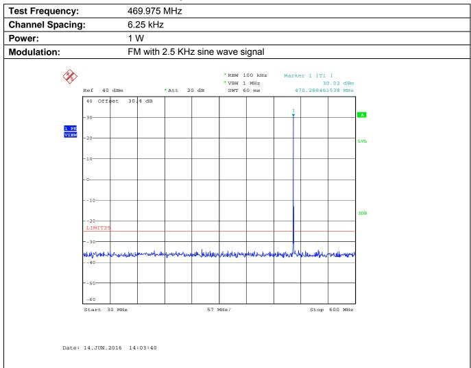
Plot 5.9.4.3.4. Conducted Transmitter Spurious Emissions for 469.975 MHz, Low Power, 600 MHz - 5 GHz
