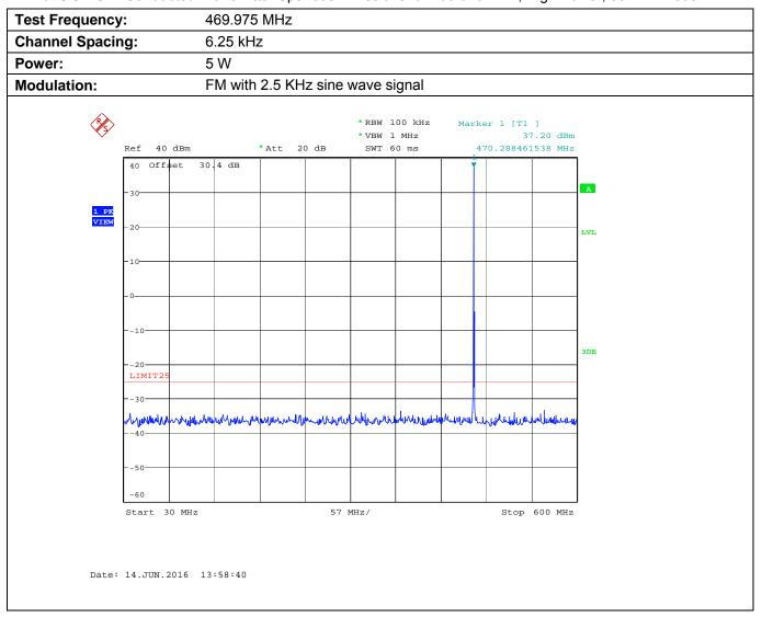
Plot 5.9.4.3.2. Conducted Transmitter Spurious Emissions for 469.975 MHz, High Power, 600 MHz - 5 GHz
