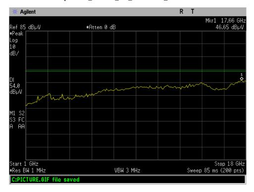
Radiated Spurious\_Band A\_FM\_1 - 18 GHz\_tuned to 30 MHz
