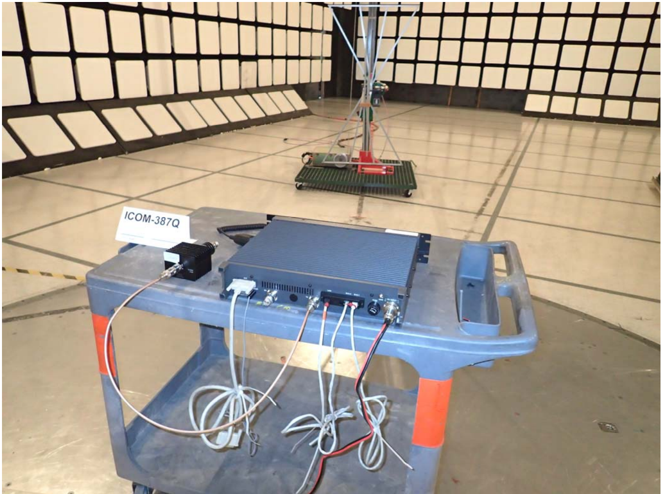
Plot #3: Tx Radiated Emission Test Setup
