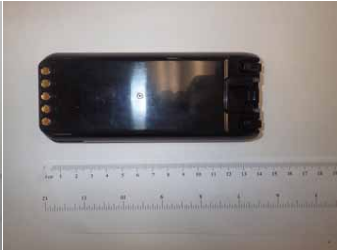
Li-ion Chargeable Battery (M/N: BP-288, 7.2V, 2200mAh)
