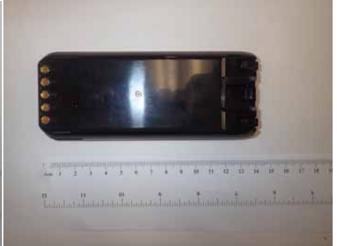
Li-ion Chargeable Battery (M/N: BP-288, 7.2V, 2200mAh)
