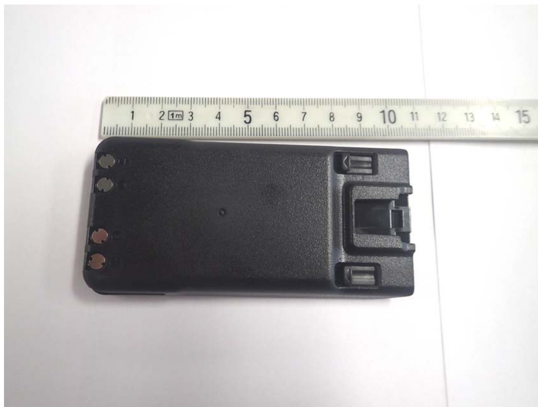
(Li-ion Chargeable Battery (M/N: BP-279 Li-ion, 7.2V, 1485mAh))
