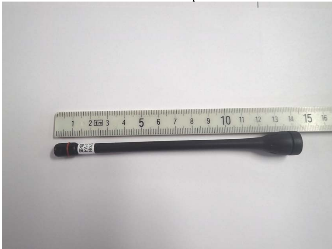
FA-SC72U 470-520 MHz Blue Tip 138mm
