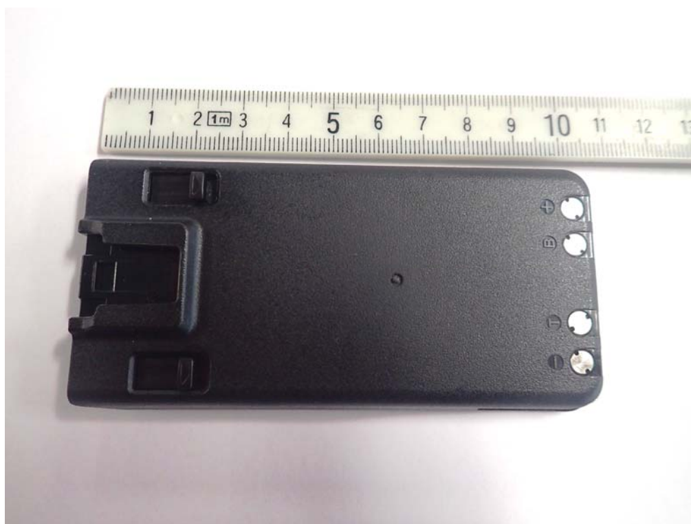
(Li-ion Chargeable Battery (M/N: BP-278 Li-ion, 7.2V, 1130mAh)
