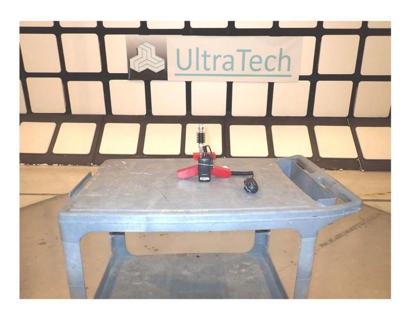
Plot #2: Tx Radiated Emission Test Setup
