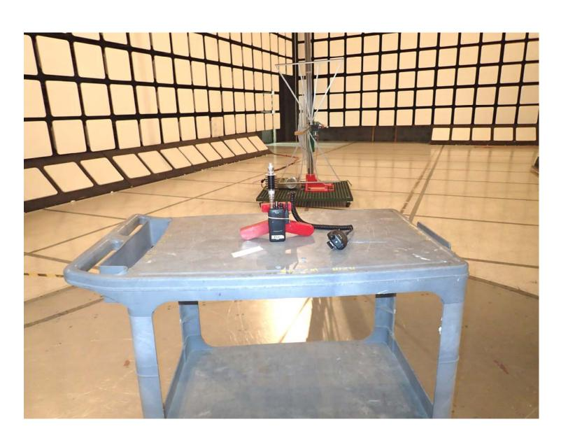
Plot #4: Tx Radiated Emission Test Setup
