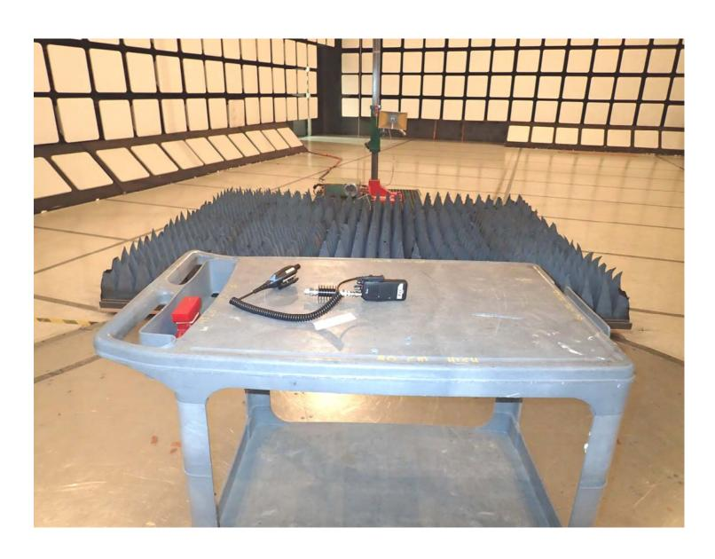
Plot #3: Tx Radiated Emission Test Setup
