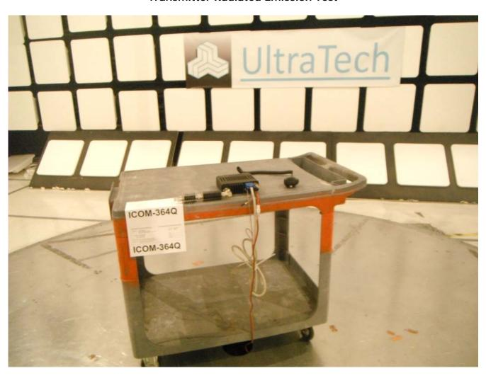
**Transmitter Radiated Emission Test**
