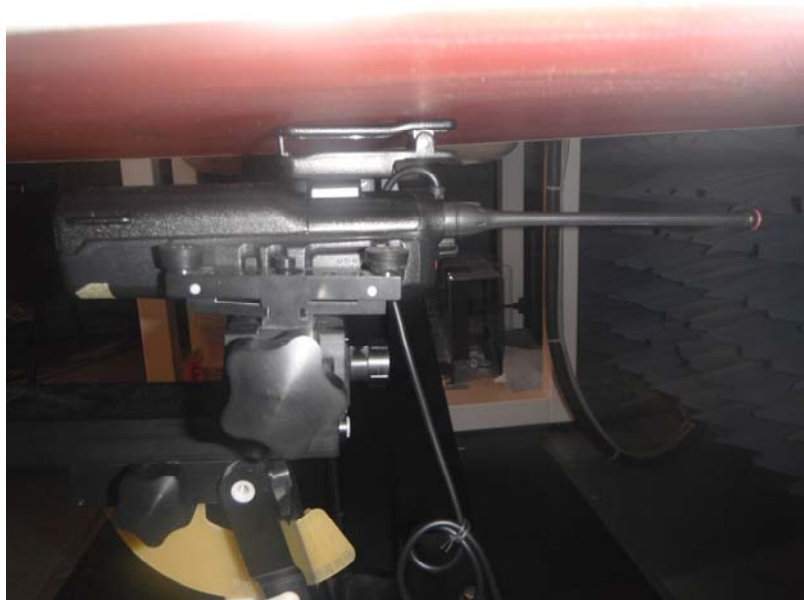
Back side of EUT in parallel to the phantom with the belt-clip (M/N: MB-93) in contact, attached HS-95 Speaker Microphone
