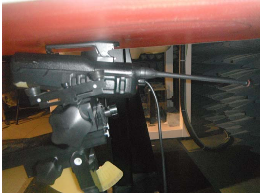
Back side of EUT in parallel to the phantom with the belt-clip (M/N: MB-94) in contact, attached HS-95 Speaker Microphone
