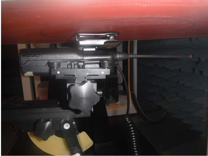
Back side of EUT in parallel to the phantom with the belt-clip (M/N: MB-93) in contact, attached HM-184 Speaker Microphone
