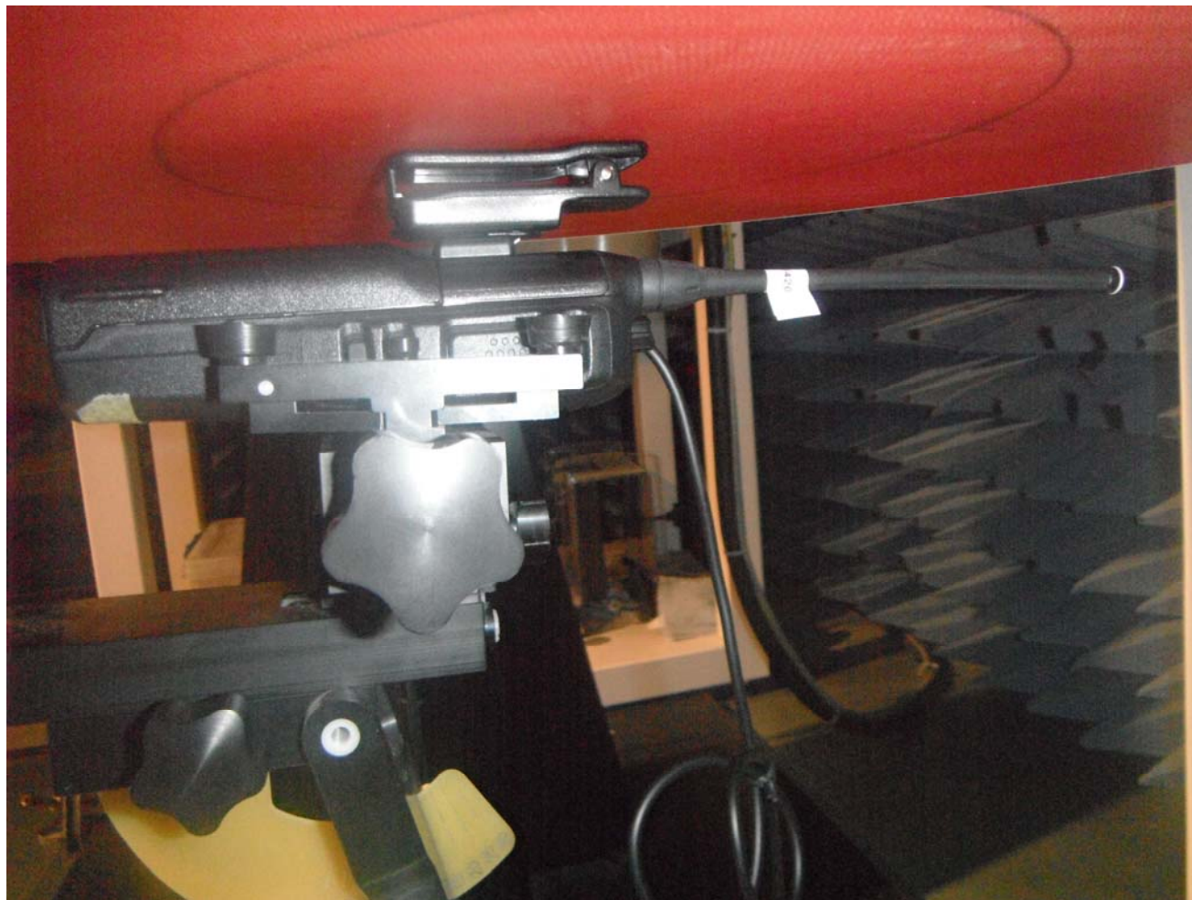
< FA-SC61UC cut antenna with the length of 156mm >
