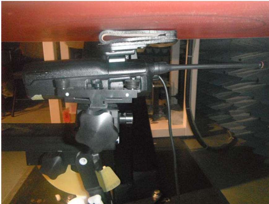
Back side of EUT in parallel to the phantom with the belt-clip (M/N: MB-94) in contact, attached HS-95 Speaker Microphone
