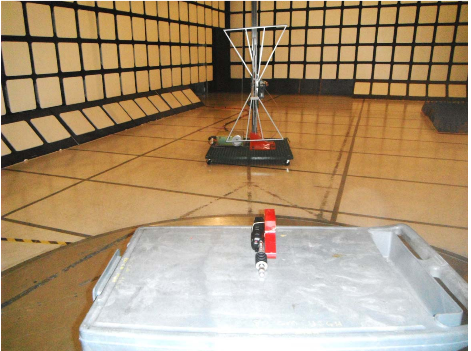
Plot #3: Tx Radiated Emission Test Setup
