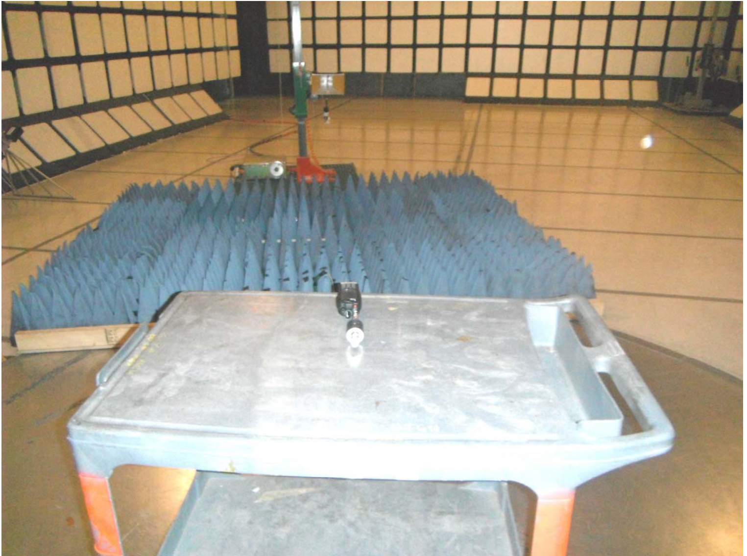
Plot #4: Tx Radiated Emission Test Setup
