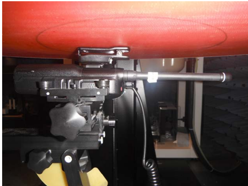
< FA-SC61VC cut antenna with the length of 133mm >
