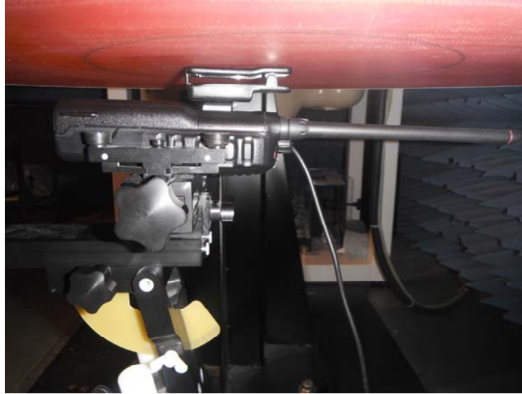
Back side of EUT in parallel to the phantom with the belt-clip (M/N: MB-93) in contact, attached HS-95
