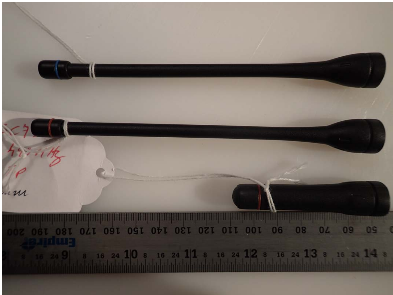
< Antenna – Blue Tip FA-SC72U 138mm, Red Tip FA-SC57U 140mm, Stubby Red Tip FA-SC73US 60mm >
