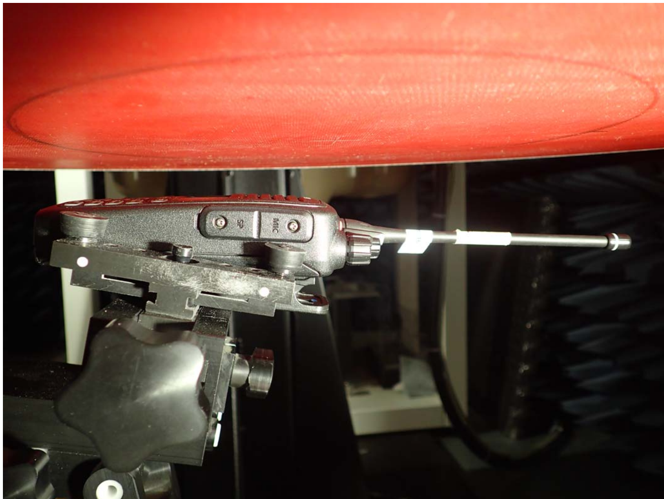
<Face Frontal Position, FA-SC61UC 144mm Cut Antenna, BP-278 battery pack>
