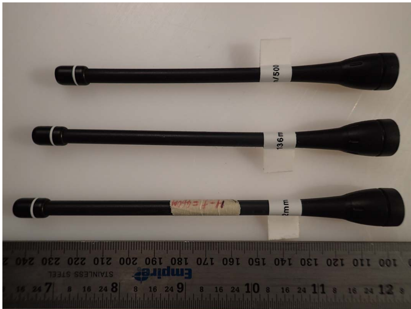
< Cut Antenna – FA-SC72FA-SC61UCU 460MHz 144mm, 480MHz 136mm, 500MHz 129mm
