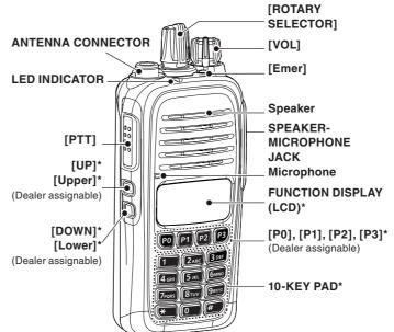
and IC-F2000 series. IC-F1000/F2000: Non-display type (Basic type)
