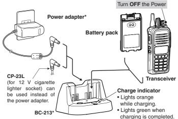
\* Not supplied, or the shape is different, depending on the transceiver version.
