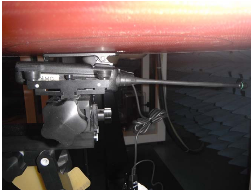
Back side of EUT in parallel to the phantom with the belt-clip (M/N: MB-133) in contact, attached HS-166LA Speaker Microphone
