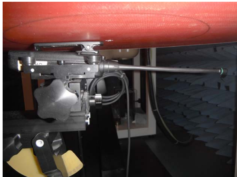
Back side of EUT in parallel to the phantom with the belt-clip (M/N: MB-133) in contact, attached HS-153LA Speaker Microphone
