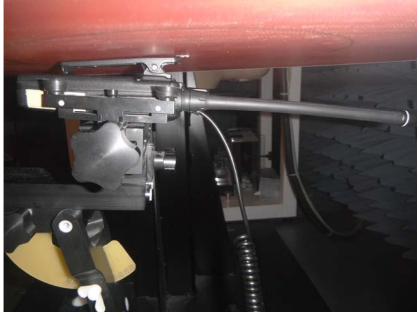
< FA-SC61VC cut antenna with the length of 174mm >
