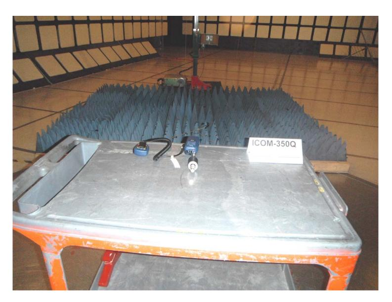
Plot #4: Tx Radiated Emission Test Setup
