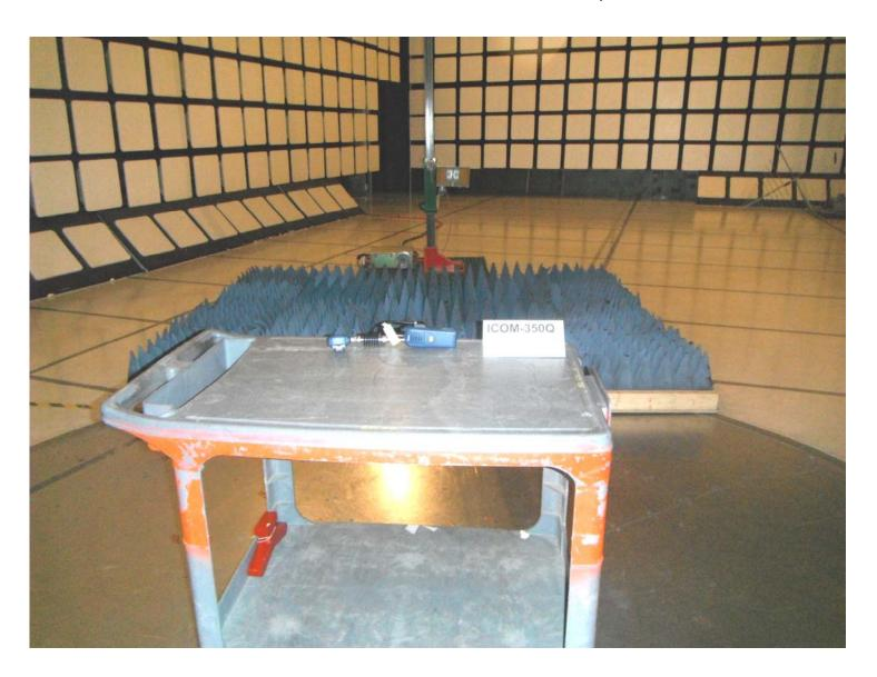
Plot #3: Tx Radiated Emission Test Setup
