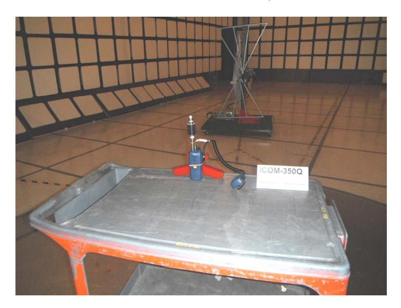
Plot #2: Tx Radiated Emission Test Setup
