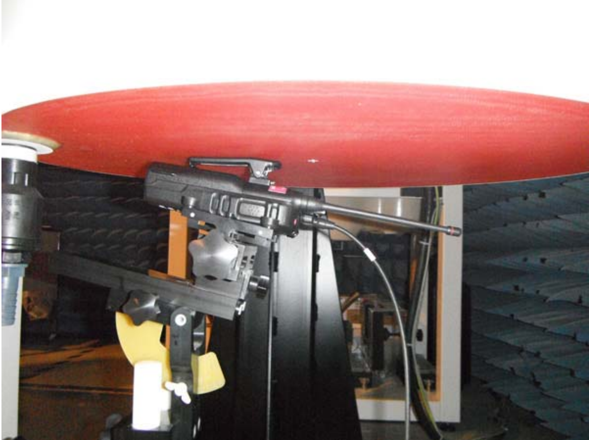
Back side of EUT in parallel to the phantom with the belt-clip (M/N: MB-94R) in contact, attached HM-184 Speaker Microphone and AD-118 ACC Adapter with V4-10001 Speaker Microphone separately
