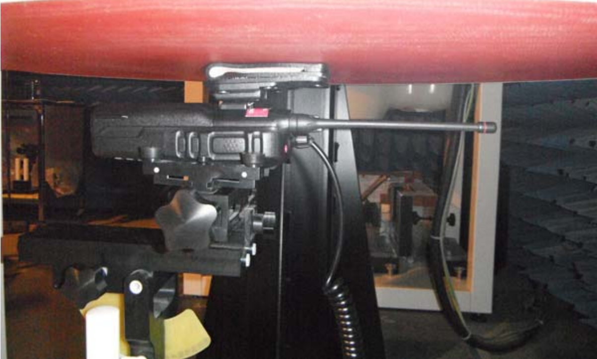
Back side of EUT, attached HM-184 Speaker Microphone, in parallel to the phantom with different types' belt-clips in contact separately
