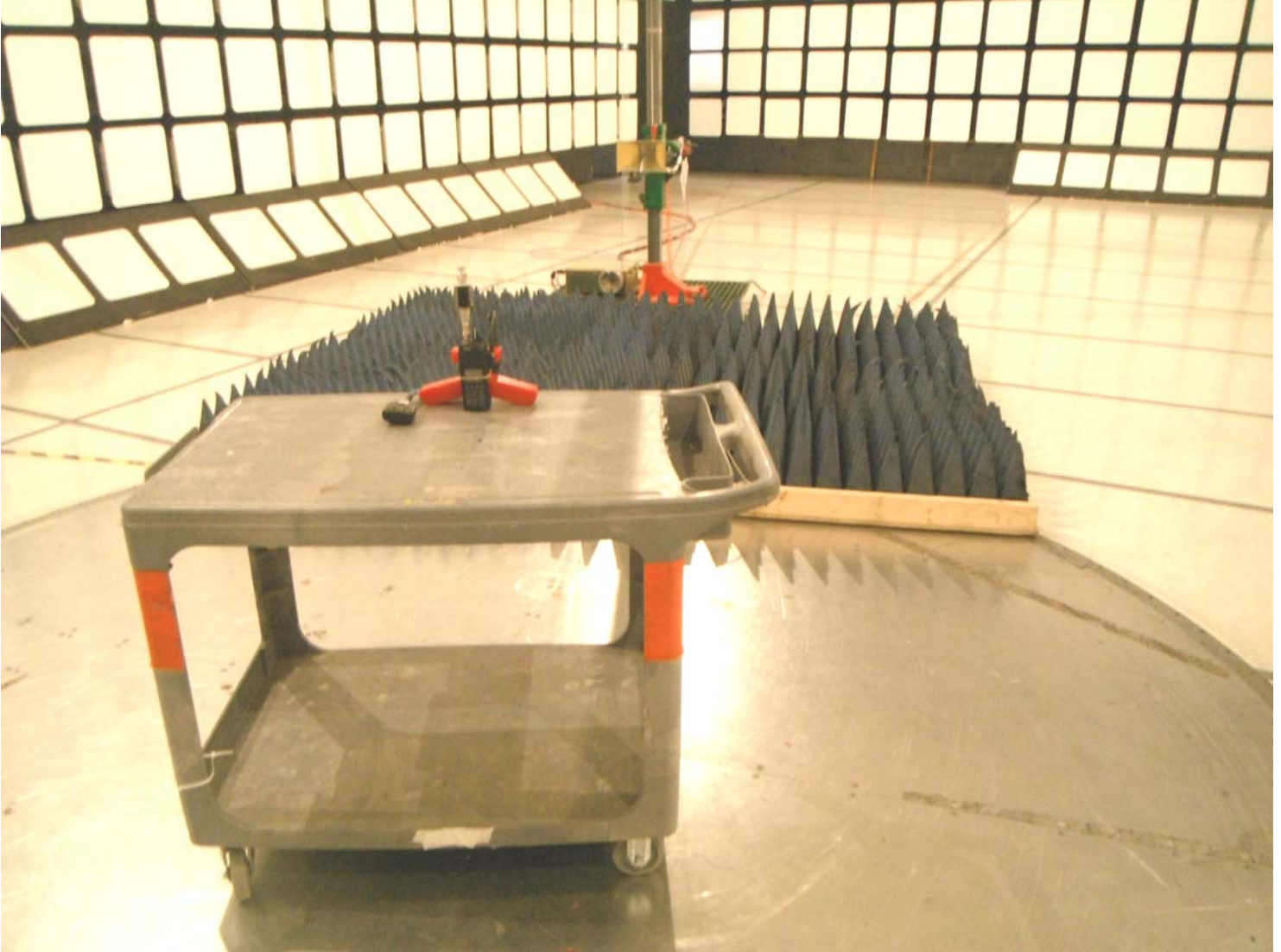
Plot #1: Tx Radiated Emission Test Setup
