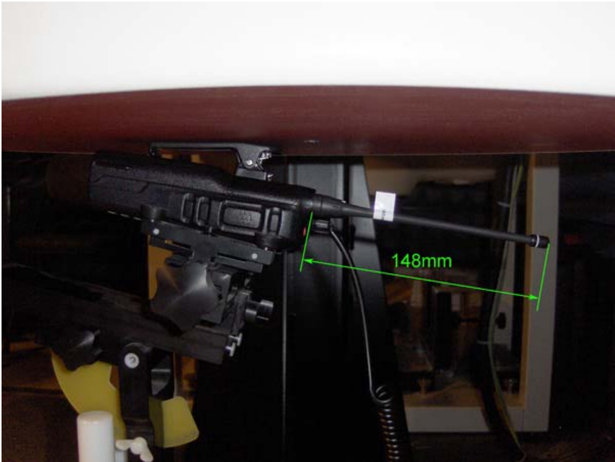
< FA-SC61UC cut antenna with the length of 148mm >
