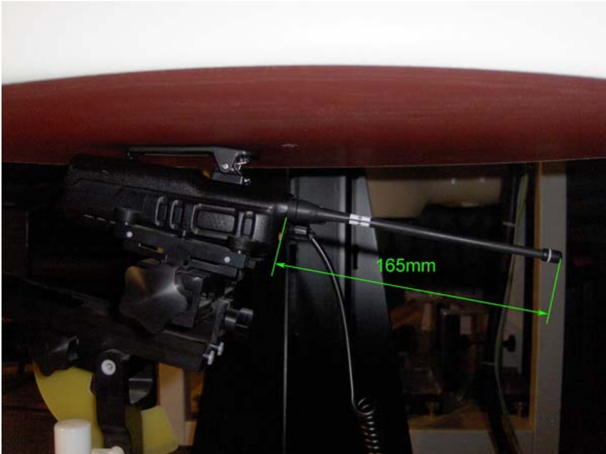
< FA-SC61UC cut antenna with the length of 165mm >
