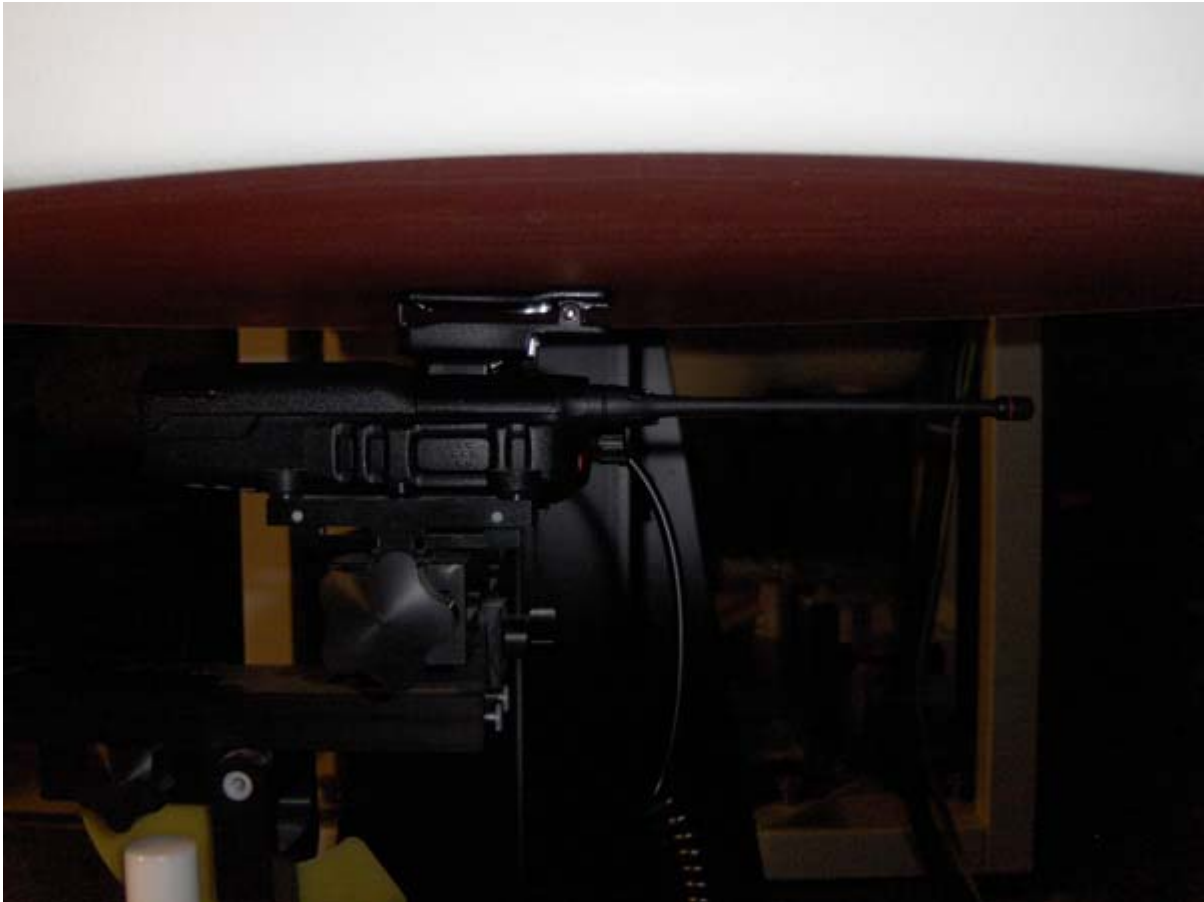
Back side of EUT, attached HM-184 Speaker Microphone, in parallel to the phantom with different types' belt-clips in contact separately
