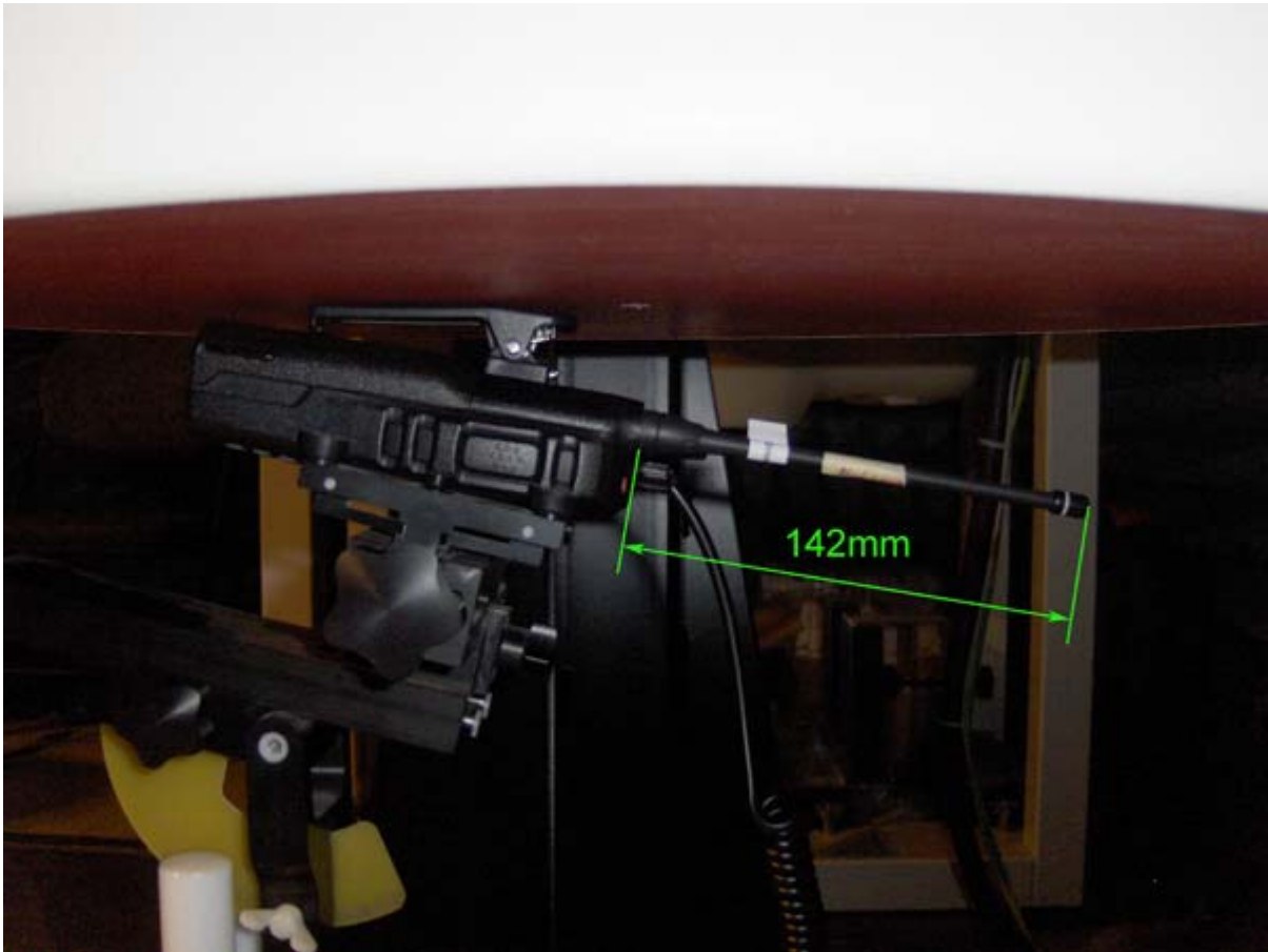
< FA-SC61UC cut antenna with the length of 142mm >
