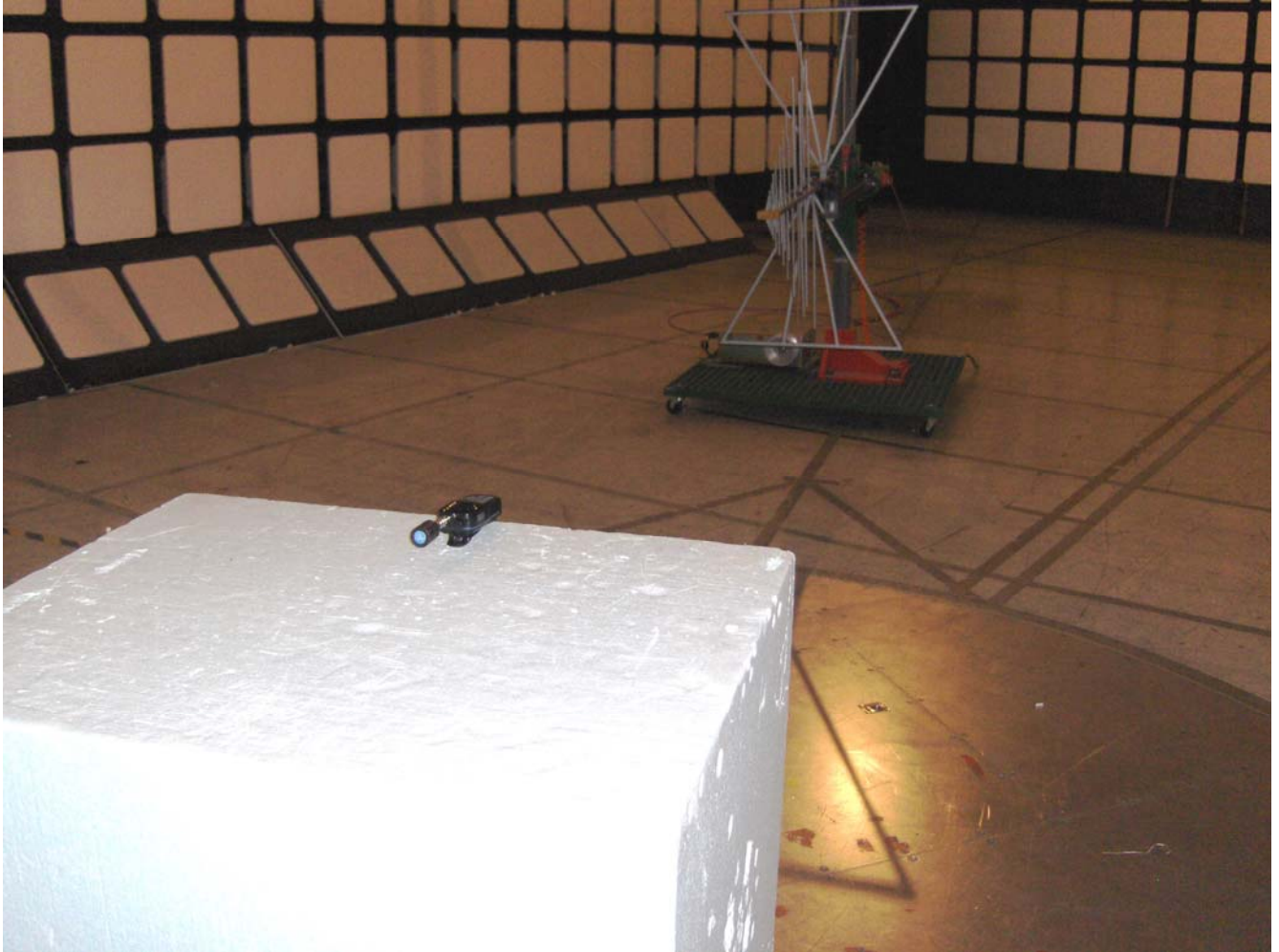
Plot #1: Tx Radiated Emission Test Setup
