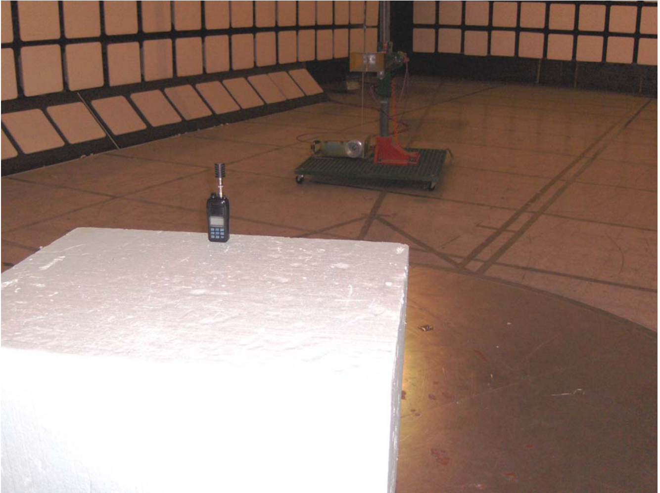
Plot #2: Tx Radiated Emission Test Setup
