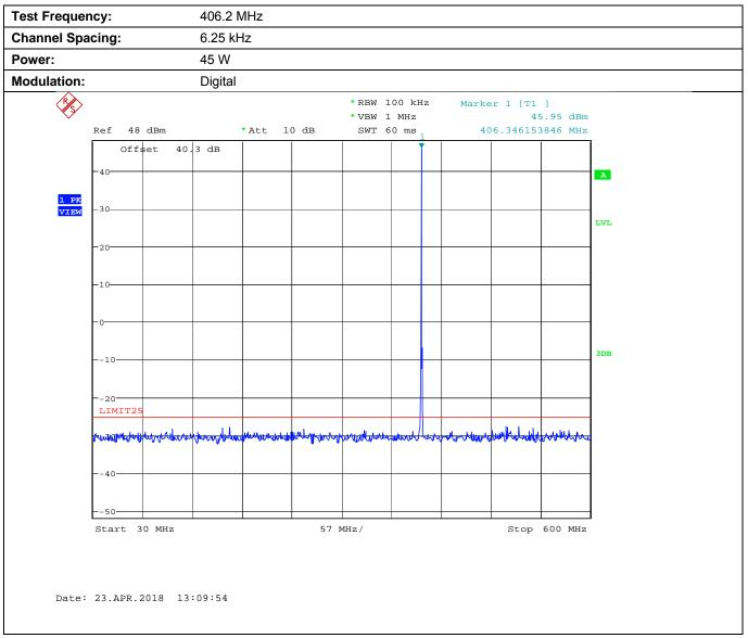
Plot 5.9.4.1.2. Conducted Transmitter Spurious Emissions for 406.2 MHz, High Power, 0.6 - 5 GHz
