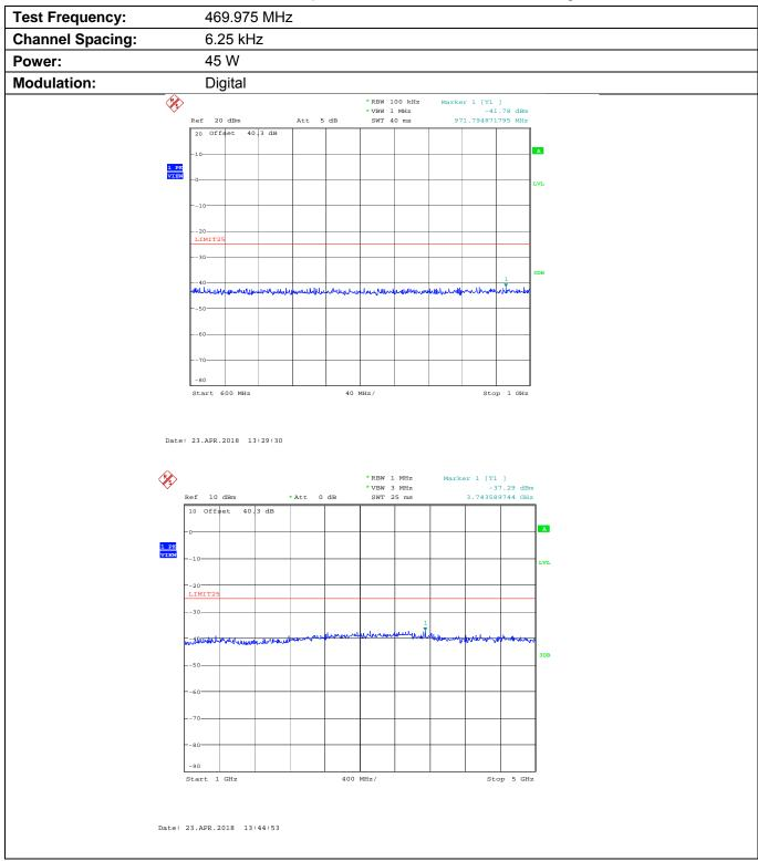
Plot 5.9.4.3.3. Conducted Transmitter Spurious Emissions for 469.975 MHz, Low Power, 30 - 600 MHz
