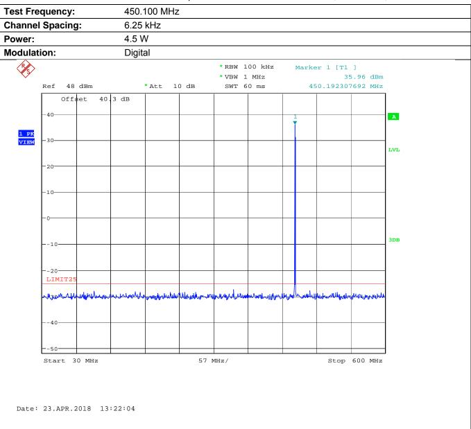
Plot 5.9.4.2.4. Conducted Transmitter Spurious Emissions for 450.100 MHz, Low Power, 0.6 - 5 GHz
