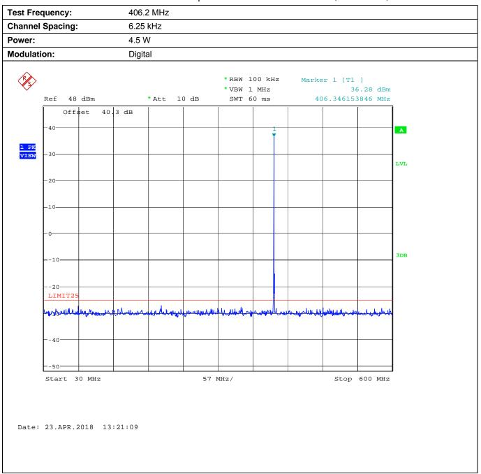
Plot 5.9.4.1.4. Conducted Transmitter Spurious Emissions for 406.2 MHz, Low Power, 0.6 - 5 GHz
