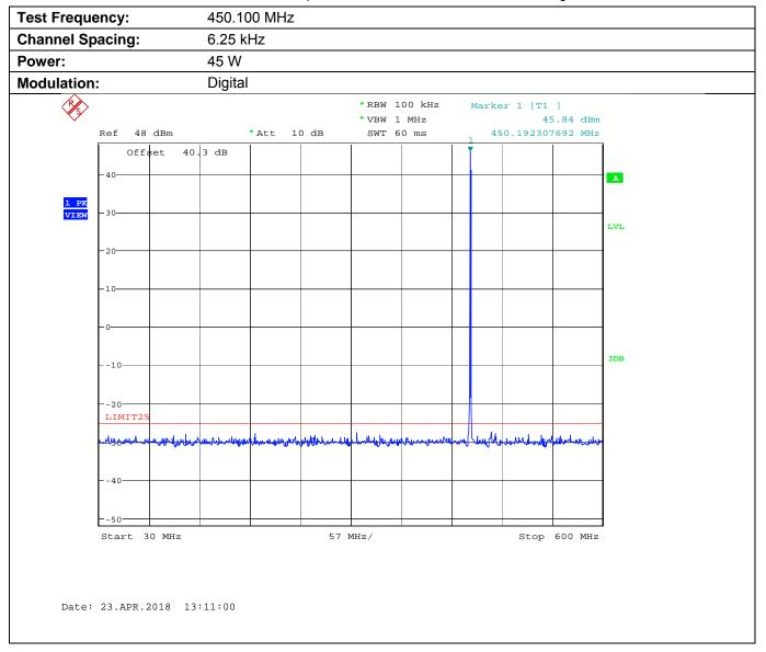
Plot 5.9.4.2.2. Conducted Transmitter Spurious Emissions for 450.100 MHz, High Power, 0.6 - 5 GHz
