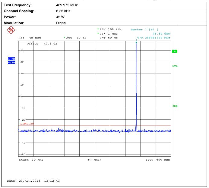
Plot 5.9.4.3.2. Conducted Transmitter Spurious Emissions for 469.975 MHz, High Power, 0.6 - 5 GHz
