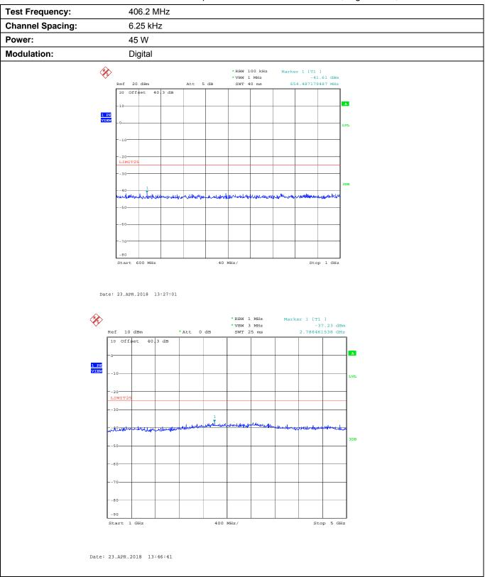
Plot 5.9.4.1.3. Conducted Transmitter Spurious Emissions for 406.2 MHz, Low Power, 30 - 600 MHz
