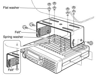
When using self-tapping screws
