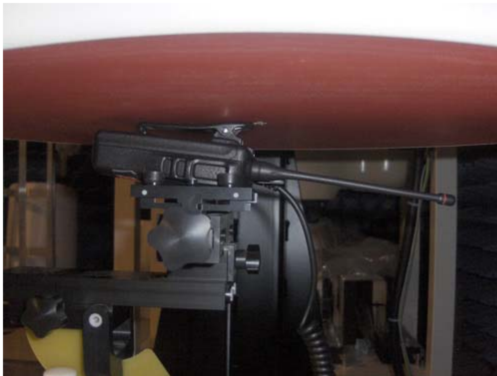
Back side of EUT in parallel to the phantom with the belt-clip (M/N: MB-124) in contact using FA-SC57U antenna; attached 3 different- type batteries separately.
