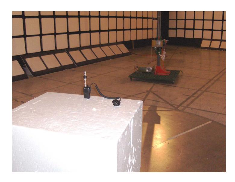
Radiated Transmitter Emission Test at 3m, Above 1GHz
