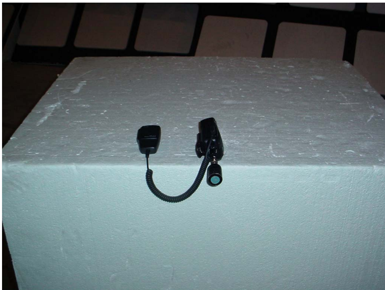
Radiated Transmitter Emission Test at 3m (Orthogonal Position 2)
