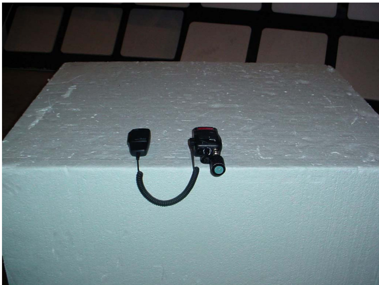
Radiated Transmitter Emission Test at 3m (Orthogonal Position 3)
