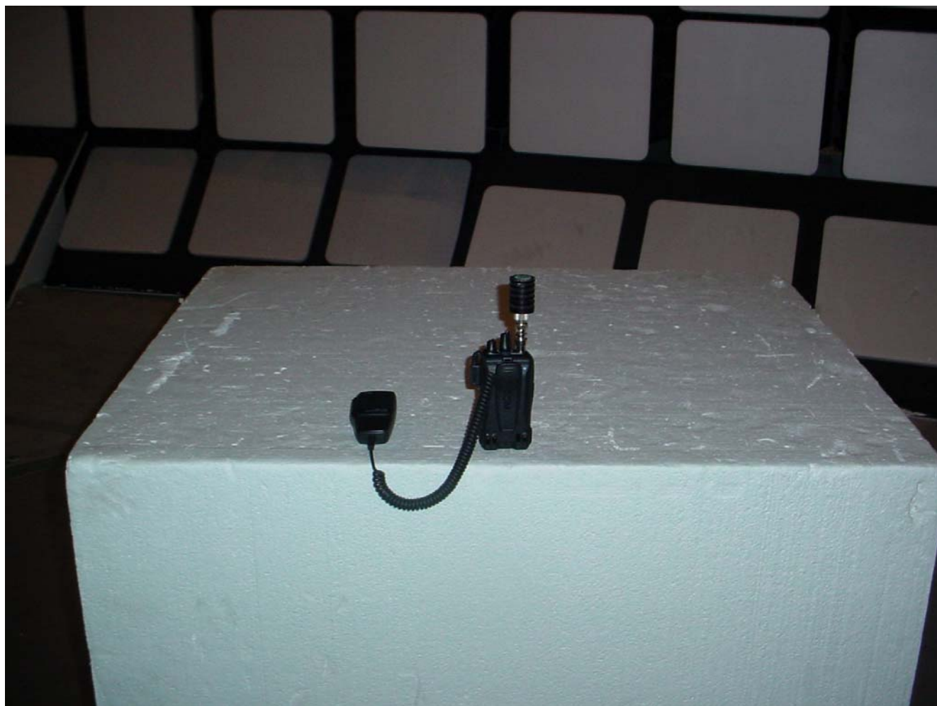
Radiated Transmitter Emission Test at 3m (Orthogonal Position 1)
