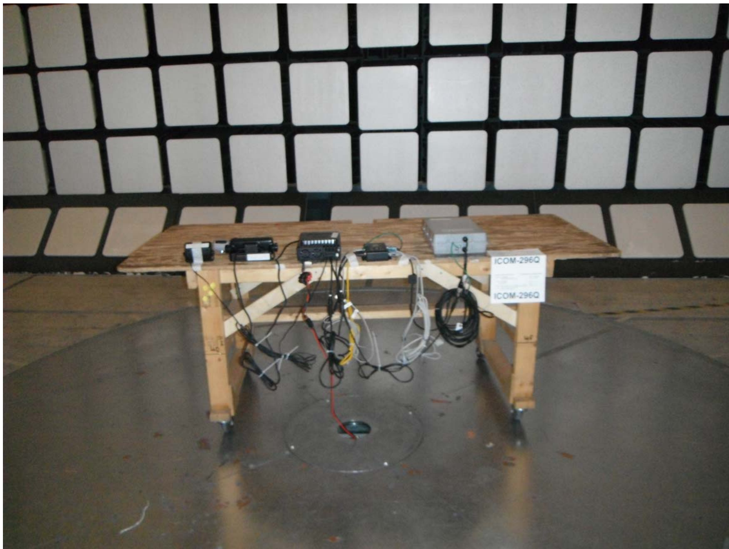
Radiated Transmitter Emission Test at 3m
