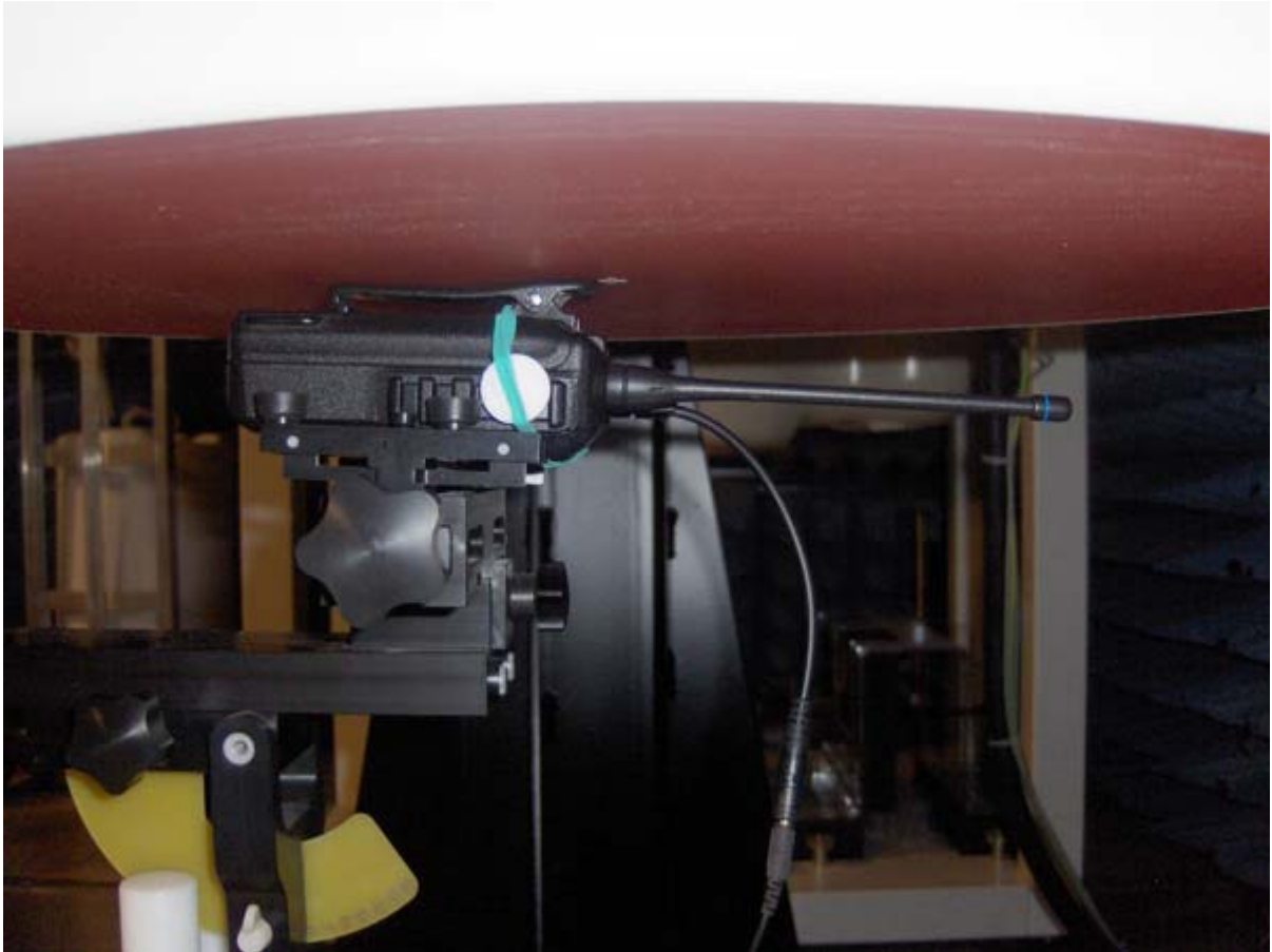
Back side of EUT in parallel to the phantom with the belt-clip (M/N: MB-124) in contact; using BP-265 chargeable battery: attached 3 different- type Speaker-microphone separately
