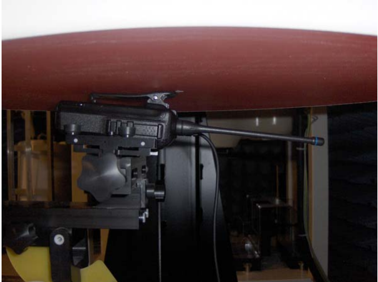
Back side of EUT in parallel to the phantom with the belt-clip (M/N: MB-124) in contact; using FA-SC72U antenna, HM153L Earphone Mic.: attached 3 different- type batteries separately.
