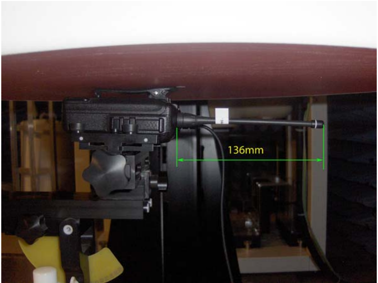
< FA-SC61UC cut antenna with the length of 136mm >
