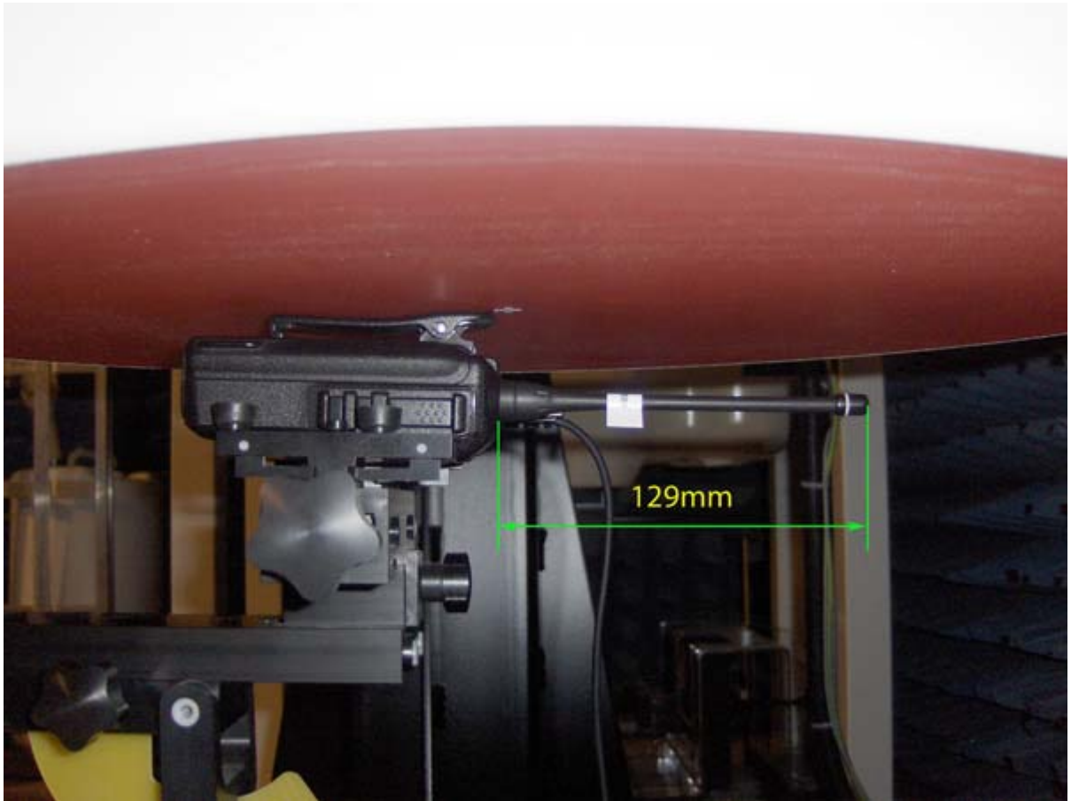
< FA-SC61UC cut antenna with the length of 129mm >
