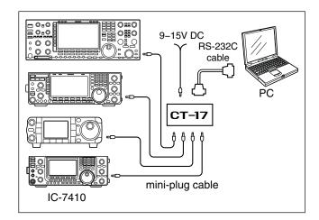
When the transceiver is connected to a PC with a USB cable (purchased separately), the optional CT-17 is not required.
