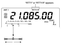
While receiving, the meter functions as the RTTY tuning meter to make correct tuning easier.
