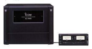
Full-duty 1 kW linear amplifier including an automatic antenna tuner. Has automatic tuning and band selection capability. Full break-in (QSK) operation is possible. The amplifier/power supply unit and the remote control unit are separated. The optional OPC-599 ADAPTER CABLE is required for connection.
