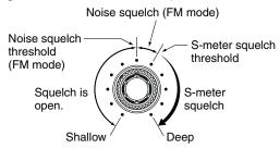
When functioning as an RF gain control (Squelch is fixed open; SSB, CW, RTTY only)
