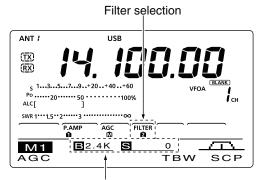
The selected filter width is displayed when [FILTER] is pushed.
