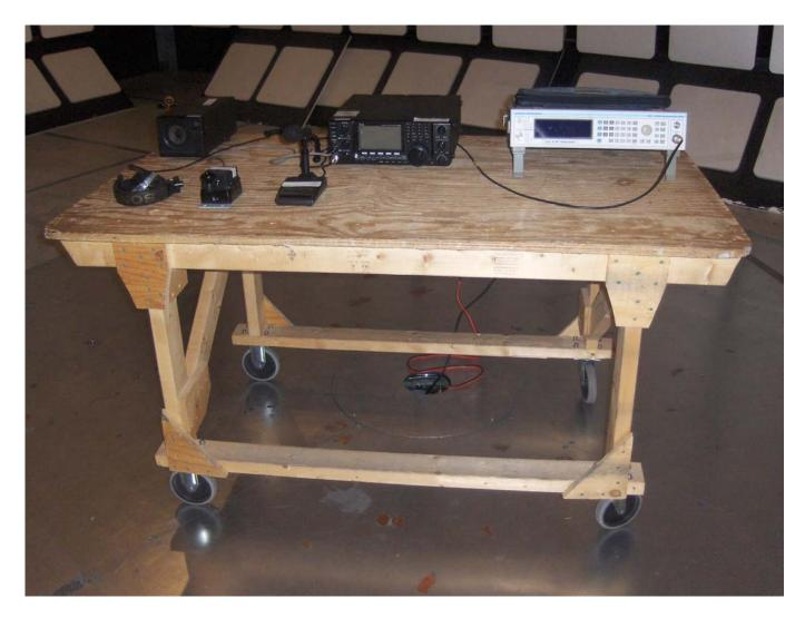
Radiated Emission at 3m Distance (Rx Mode)
