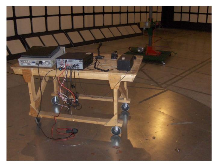
Radiated Emission at 3m Distance (Digital Device)
