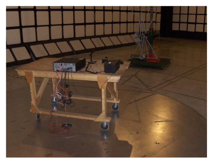
Radiated Emission at 3m Distance (Digital Device)
