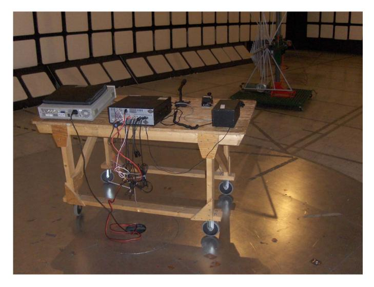
Radiated Emission at 3m Distance (Rx Mode)
