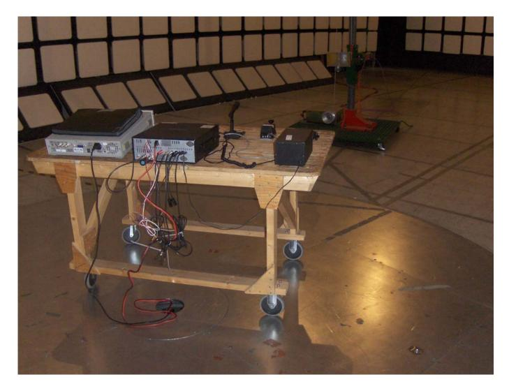
Radiated Emission at 3m Distance (Rx Mode)
