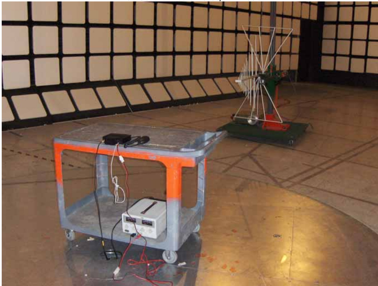
< Radiated emission test, Rx mode >
