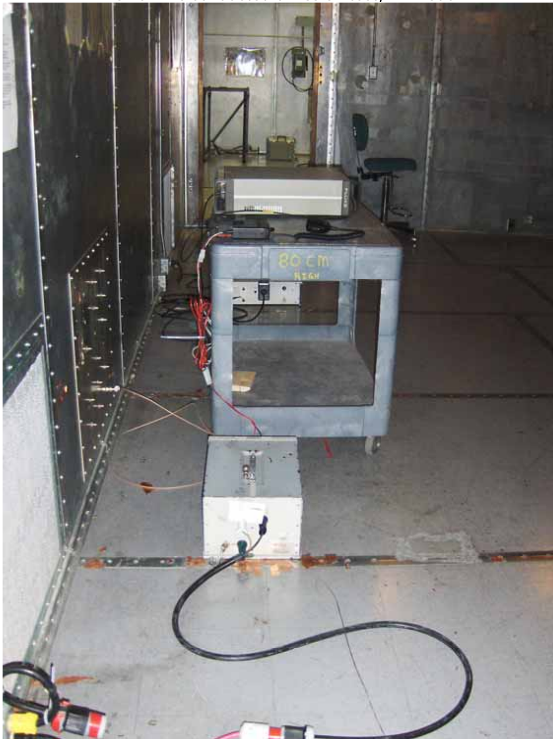
< Power line conducted emission test, Rx mode >
