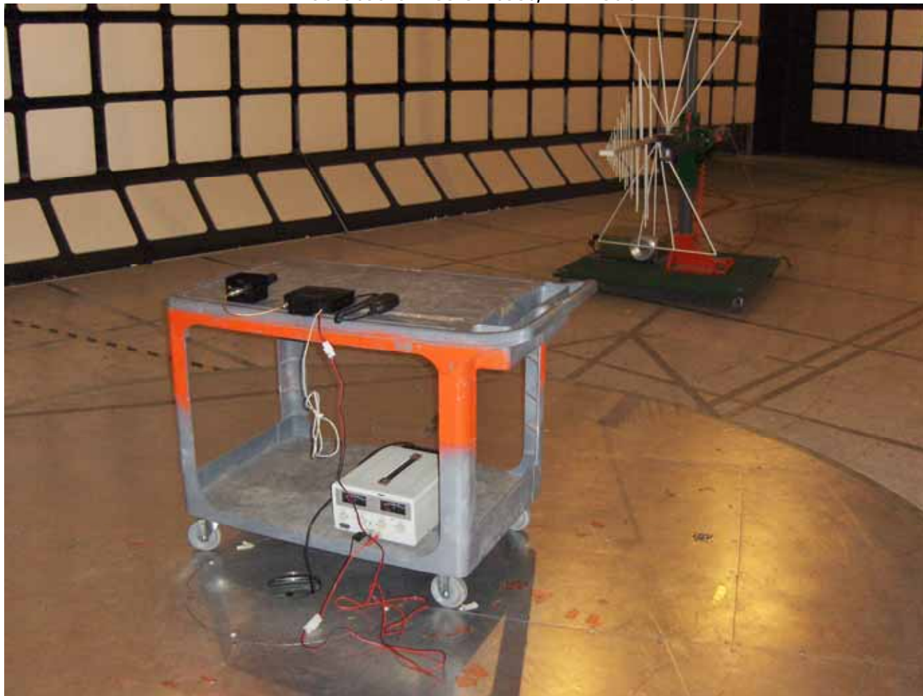
< Radiated emission test, Tx mode >
