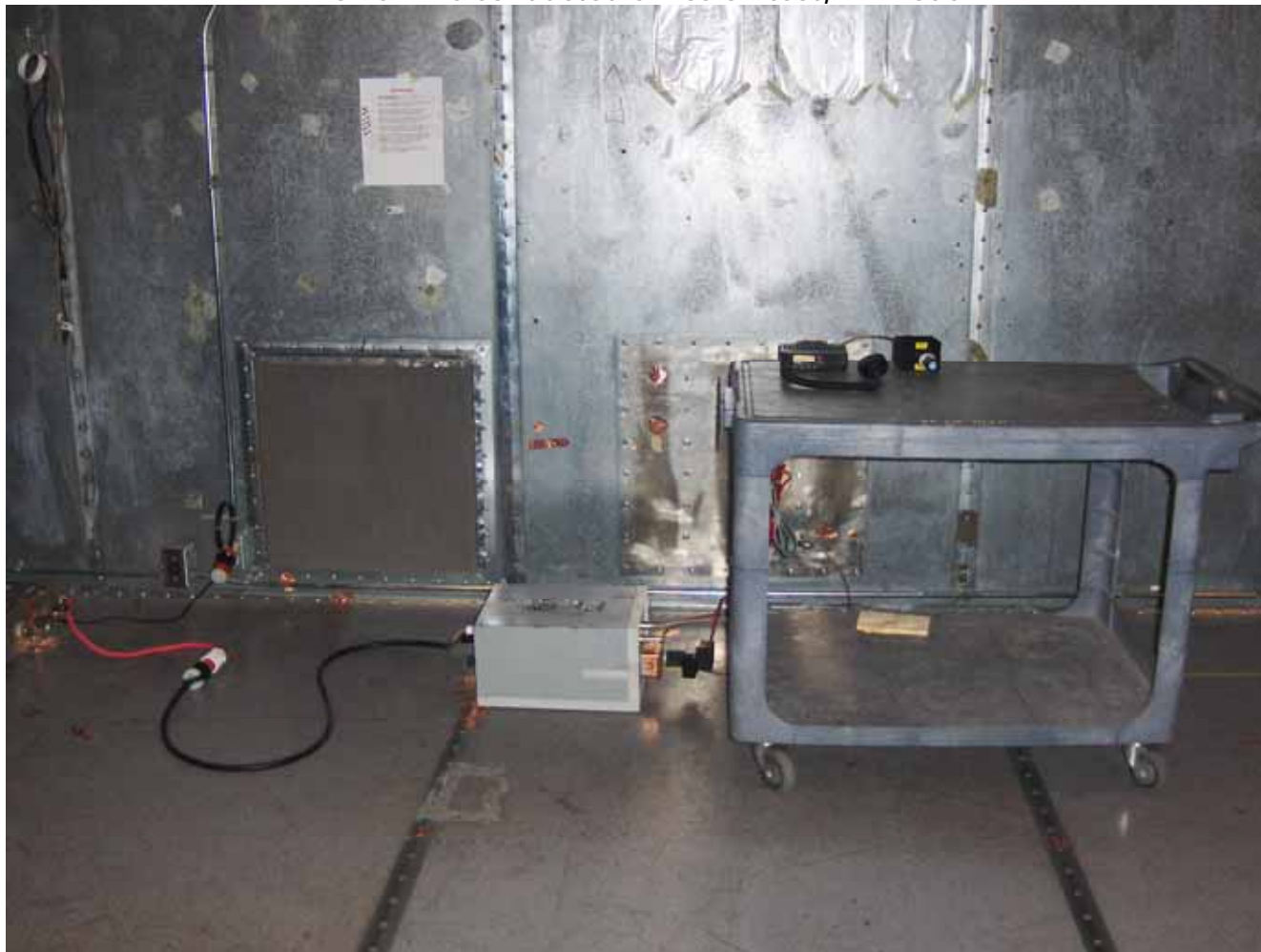
< Power line conducted emission test, Tx mode >
