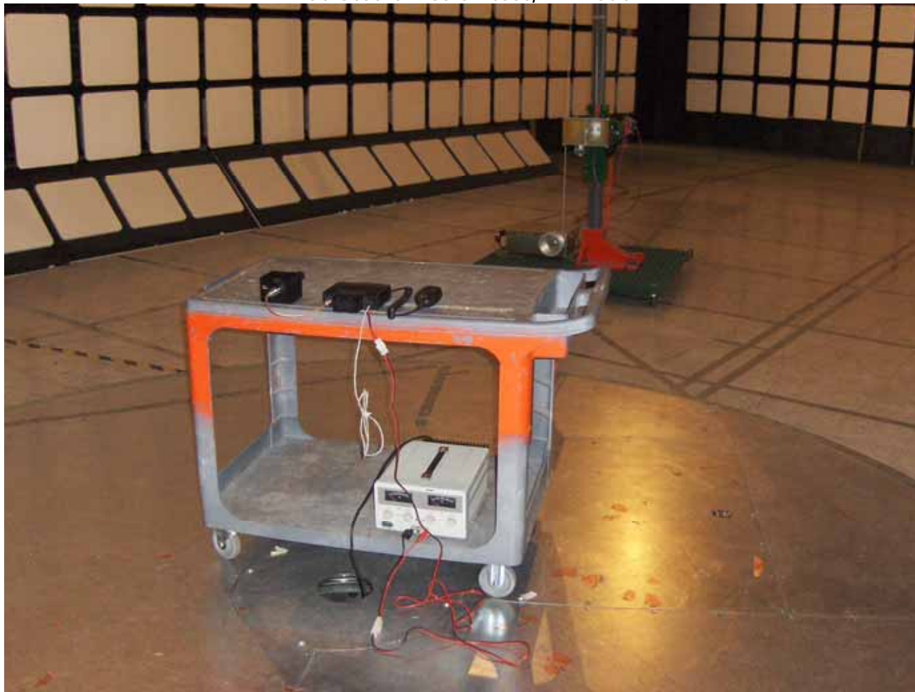
< Radiated emission test, Tx mode >
