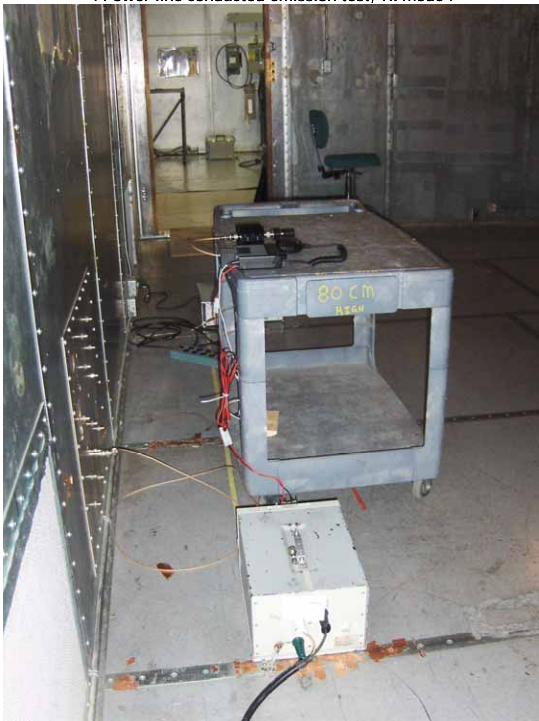
< Power line conducted emission test, Tx mode >
