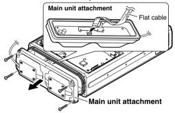
⑤ Unscrew the 4 screws, then remove the front plate from the main unit attachment. Then unscrew the circuit board screw, and disconnect the separation cable, if it is connected.
