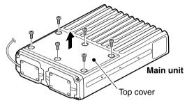
3 Unscrew the screw that is attached to the chassis.
