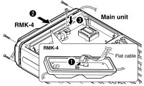
③ Replace the top cover and 6 top screws removed in step② in p. 1, then reconnect the DC power cable.
