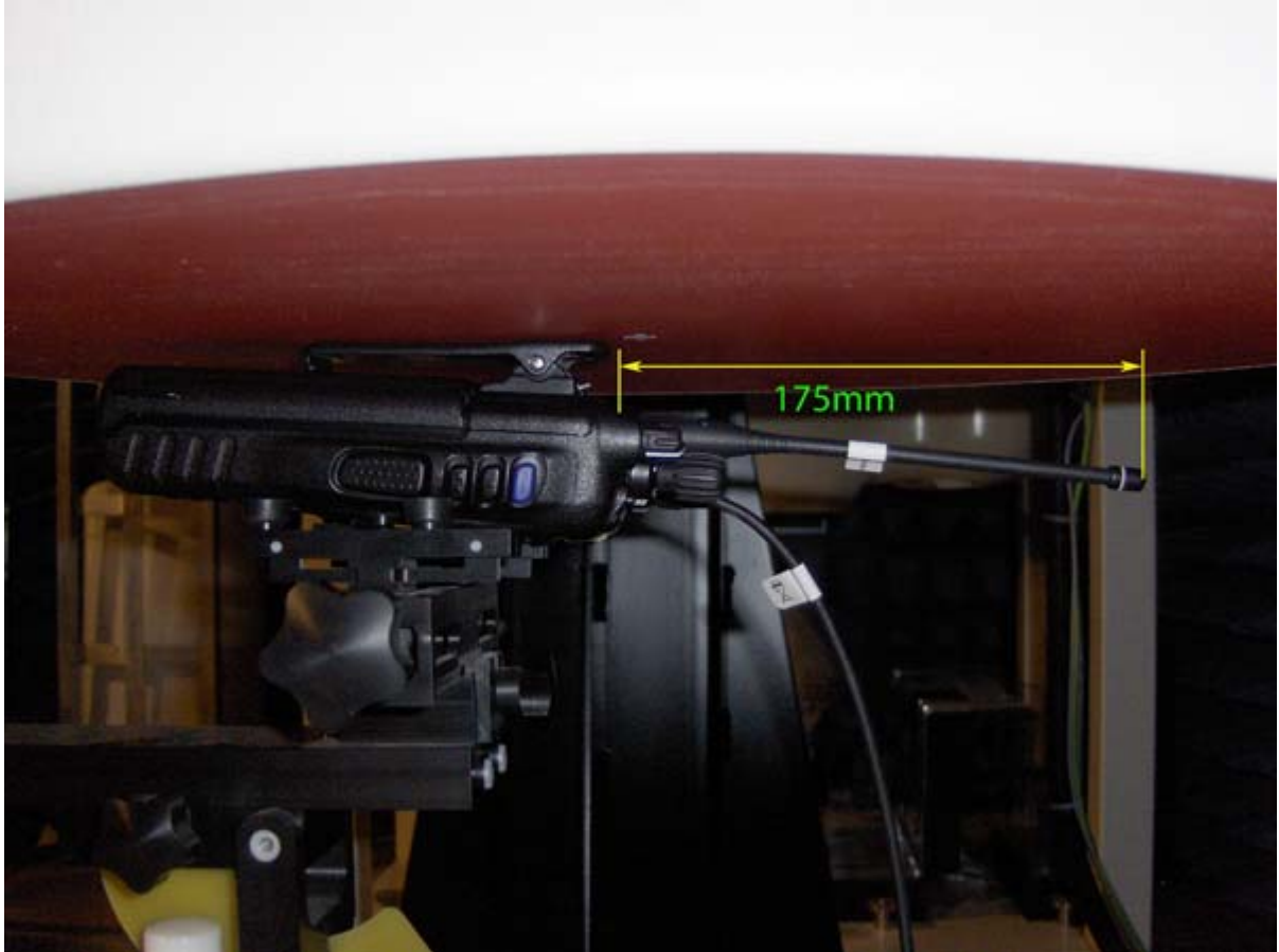
< FA-S76UC cut antenna with the length of 175mm >
