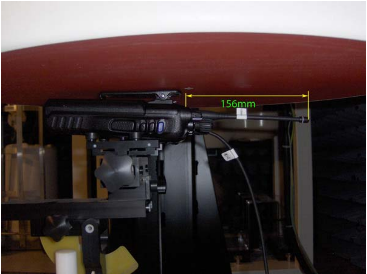
< FA-S76UC cut antenna with the length of 156mm >
