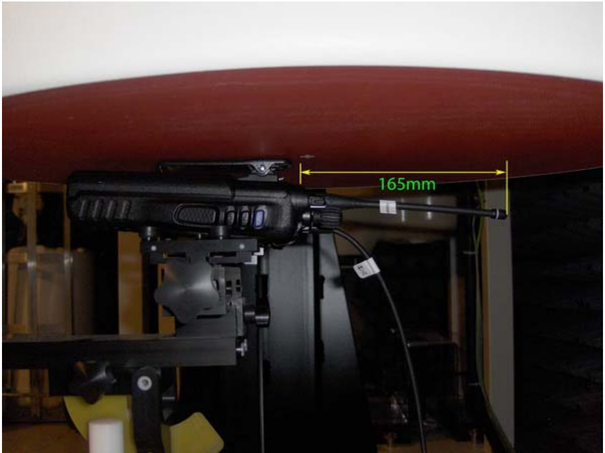
< FA-S76UC cut antenna with the length of 165mm >
