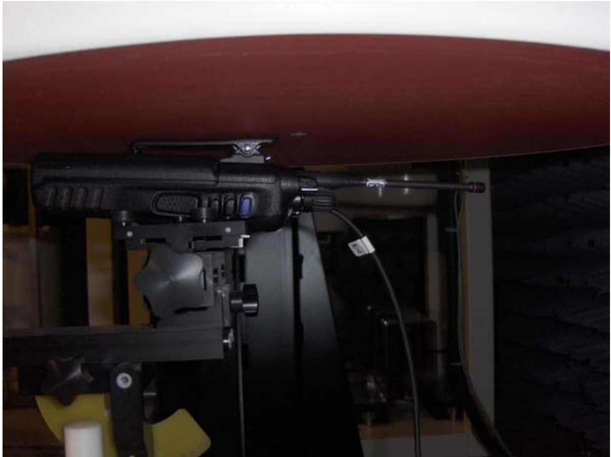
Back side of EUT in parallel to the phantom with the belt-clip (M/N: MB-115) in contact; using FA-S58U antenna and BP-254 chargeable battery: attached 3 different- types accessories separately.
