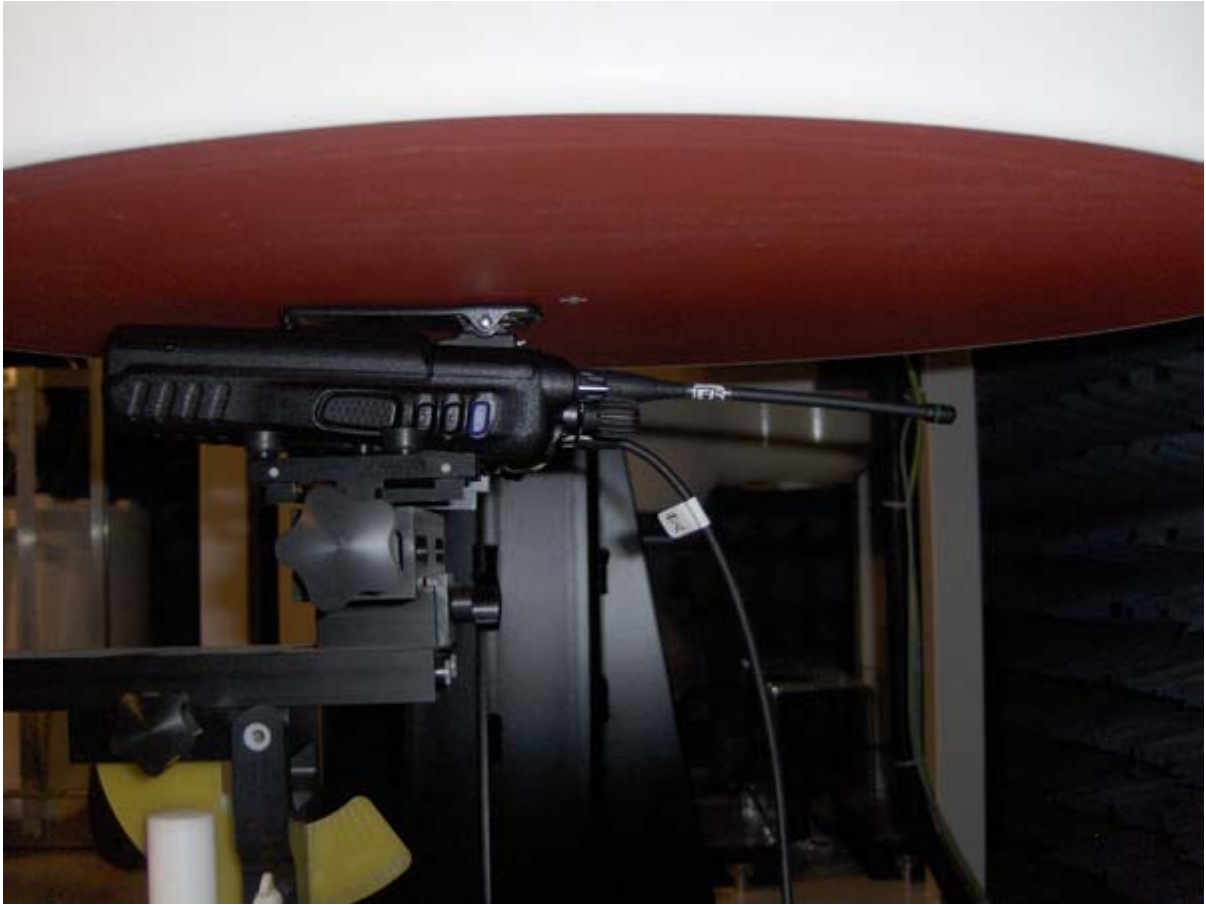
Back side of EUT in parallel to the phantom with the belt-clip (M/N: MB-115) in contact; using FA-S30U and BP-254 chargeable battery: attached 3 different- types accessories separately.
