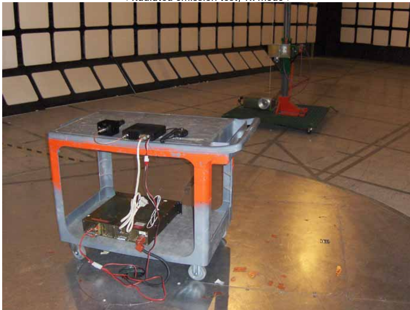
< Radiated emission test, Tx mode >
