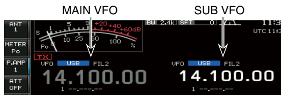
Access to SUB VFO
