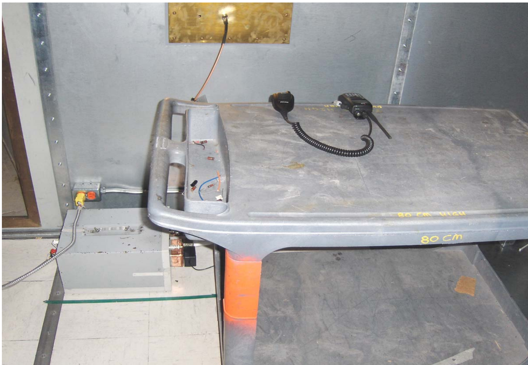
Photo #2: AC Powerline Conducted Emissions
