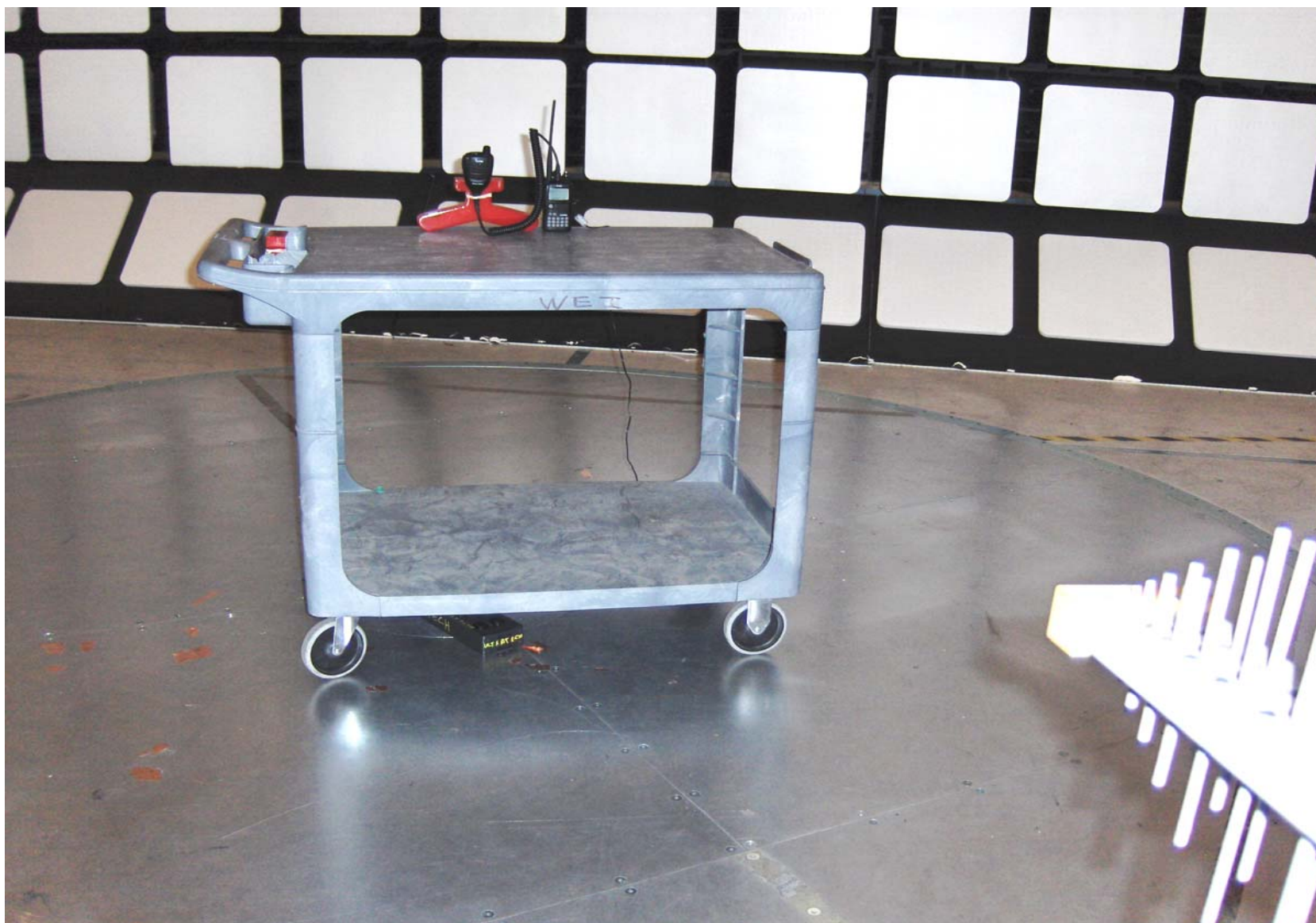
Photo # 6: Radiated Emissions at 3 meters
