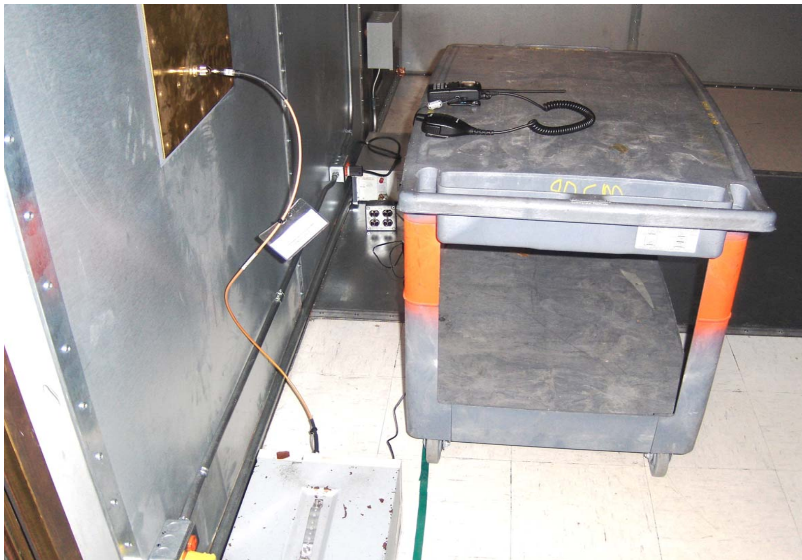
Photo #1: AC Powerline Conducted Emissions
