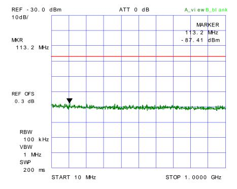
The emissions were scanned from 30 MHz to 1.0 GHz and all emissions found were more than 20 dB below the limits.
