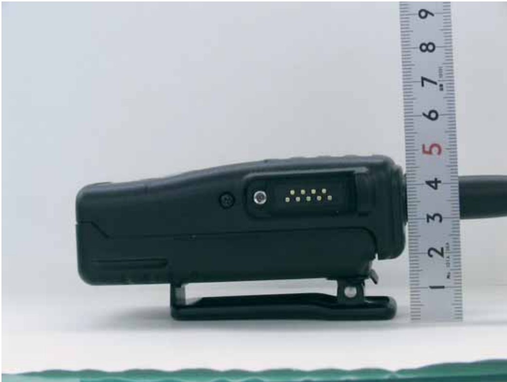
Pic.#1 Distance from the antenna with the thinnest belt-clip (M/N: MB-98) mounted
