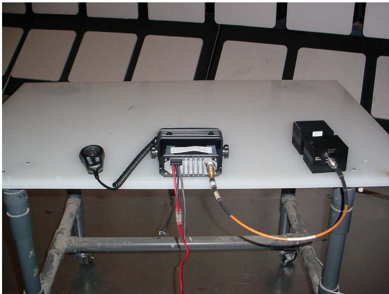
Plot #2: Radiated Emission Test Setup
