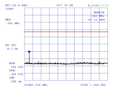
Carrier Frequency (MHz): 156.050 Power (dBm): 28.51 Limit (dBc): 41.51
